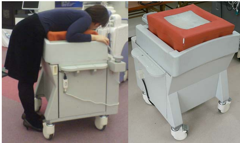
Figure 1. The prototype full-breast scanner ASU-1004 (right) with a patient in prone position (left).
