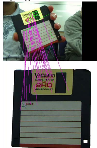
Fig. 3: SIFT feature matching in action. The reference image (below) is located within the camera frame (above) by locating common key points, connected by lines.
