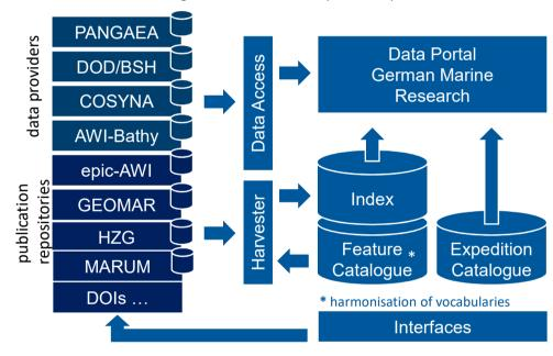
The portals architecture integrates and enables the search of distributed content from our data providers. Procedures for harvesting and indexing of metadata are based on ,elasticsearch' Cluster of Apache Lucene.
