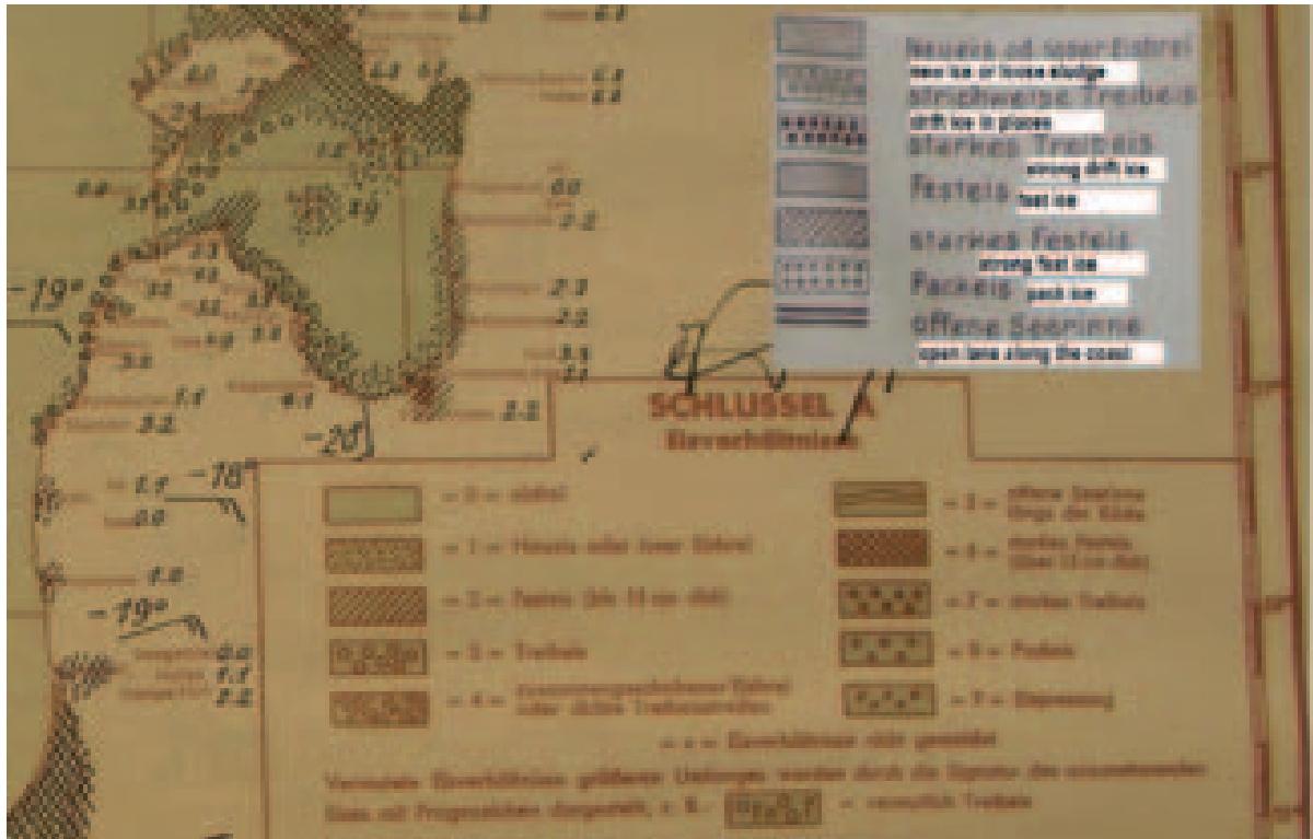
Fig 3 Section of German ice chart of 25.01.1943 (Deutsche Seewarte) 1 showing the symbols (valid from 1934/35-1953/54) related to the 1 st Baltic Ice Code (English version see above) with part of the Baltic coast and the Gulf of Riga. For comparison the symbols valid from 1927/28-1933/34 are inserted.
