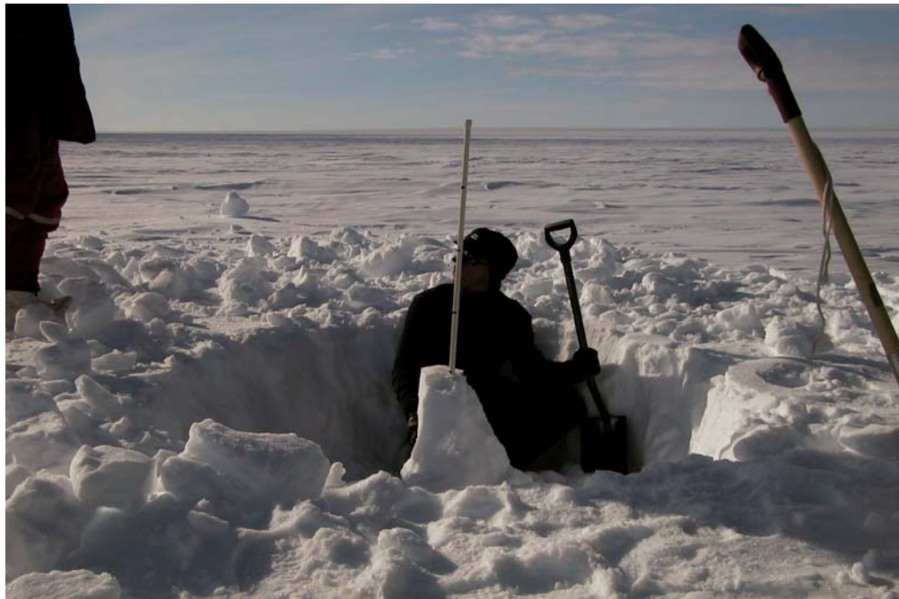
Figure 28. The sensor part of the automatic snow sensor was dug out and pipe attached them was then easy to pull out. (Photograph by E. Kärkäs)
