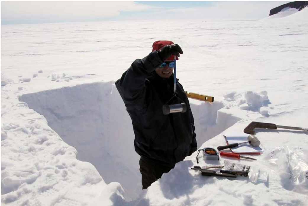
Figure 11. Snow samples were weighed with a spring balance. (Photograph by K. Kanto)
