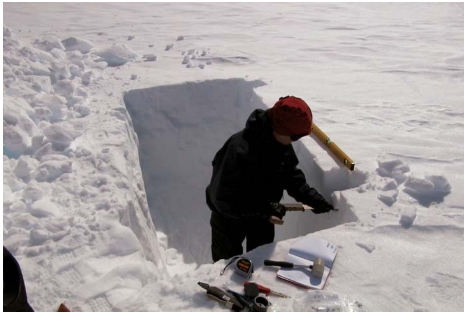
Figure 9. Snow properties were measured from the wall of the snow pit. (Photograph by K. Kanto)
