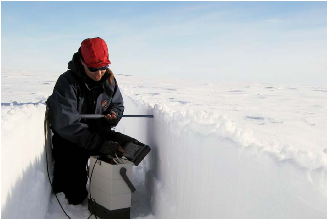
Figure 12. The snow fork measures the dielectric constant of snow. (Photograph by K. Kanto)
