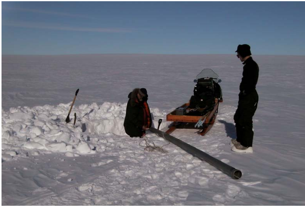
Figure 27. The batteries were used as a power supply in snow sensors and they were packed in a 4 meter pipe. (Photograph by E. Kärkäs)
