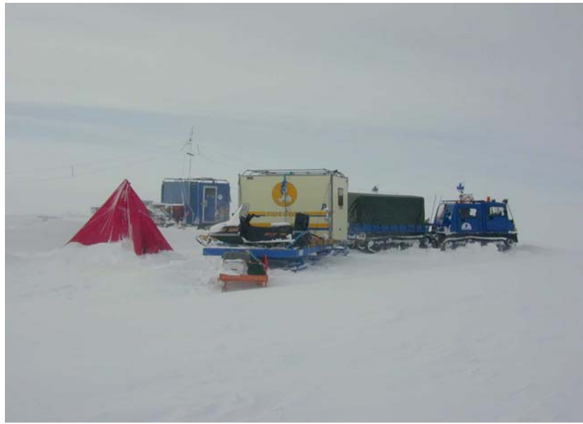
Figure 6. A heavy portable fieldcamp consisting of two survival modules on sledges pulled by articulated tracked vehicles. The red Scott-tent was used as a toilet. (Photograph by H. Granberg)
