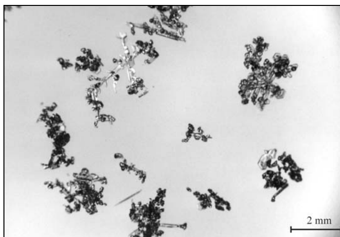
Figure 20. Surface grains from the site 1 in 2000/2001. Forms of stellar shape crystals are still visible. (Photograph by E. Kärkäs)
