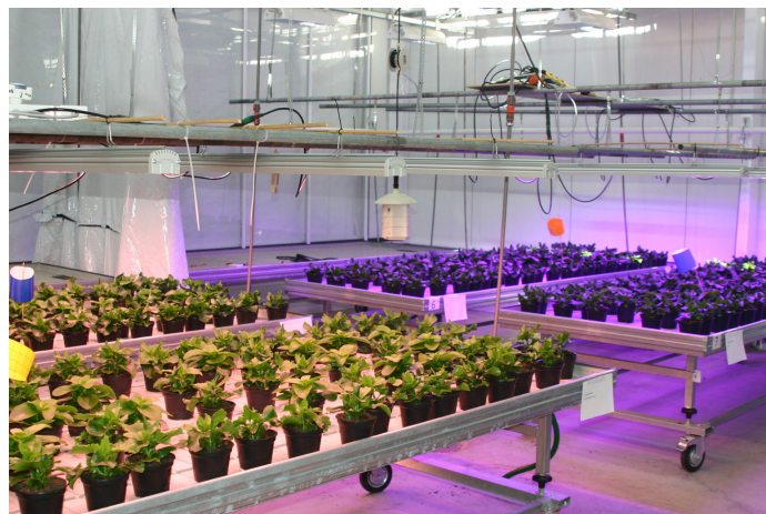
Figure 4.3: A comparison of the performance of two types of LED lamps with different emission spectra being used for the cultivation of an ornamental species ( Kalanchoe ). Photograph: © Valoya Oy.
