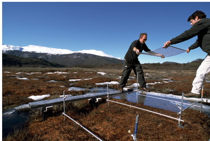
Figure 2.24: Filters in the field, stretched between two metal rods. By rolling the film onto the rods, it can be kept under tension. The researchers are standing on wooden catwalks used for access to the plots. Ushuaia, Argentina. Photograph: Kevin Maloney.
