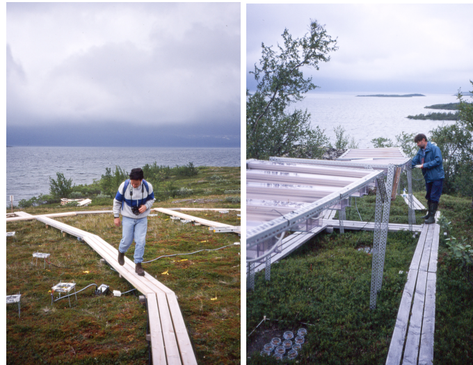
Figure 4.9: View of two UV-B experiments in Abisko, Sweden, showing the use of catwalks to protect the natural vegetation under study. Left: use of small UV-B lamps on small plants; Dr. Carlos L. Ballaré. Right: Use of frames with 40W UV-B lamps; Prof. Lars Olof Björn. Photographs: Pedro J. Aphalo.
