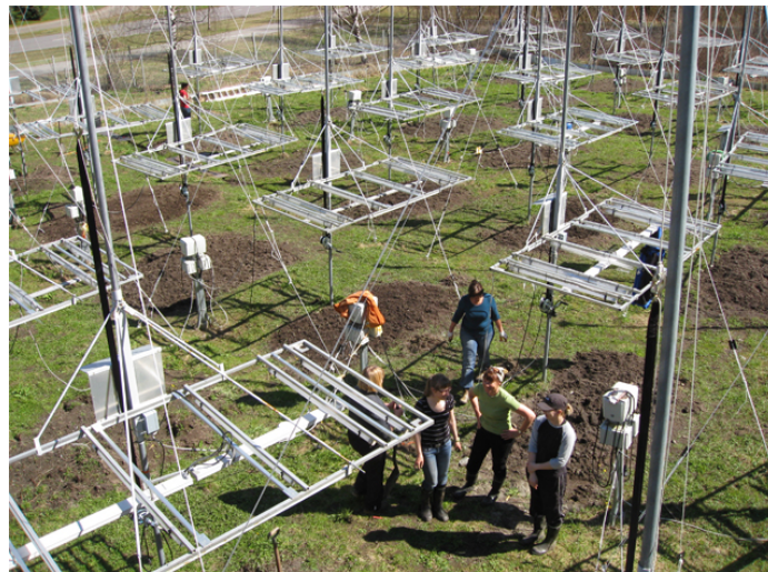
Figure 2.17: Modulated UV-B supplementation system in Joensuu in 2012. The new design of the support reduces shading. Infrared heating has been added along the middle of the frames. Photo: Matti Savinainen
