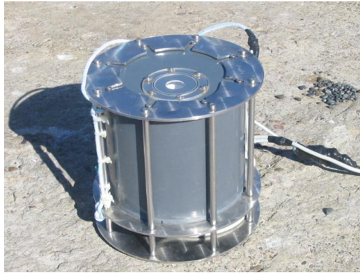
Figure 3.21: Underwater Eldonet (European light dosimeter network). (Photograph by Donat Häder, reproduced with permission.)
