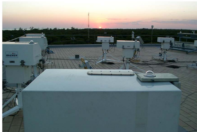
Figure 3.15: Brewer spectroradiometers participating in a measurement campaign in Huelva, Spain, in October 2005. Photograph: Anu Heikkilä.
