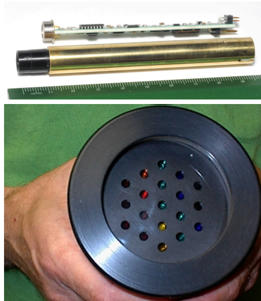
Figure 3.11: Top: microradiometer used in multichannel instruments from Biospherical Instruments; bottom: radiance fore-optics of a PRR-800 radiometer with 19 channels. Photographs © by Biospherical Instruments Inc.
