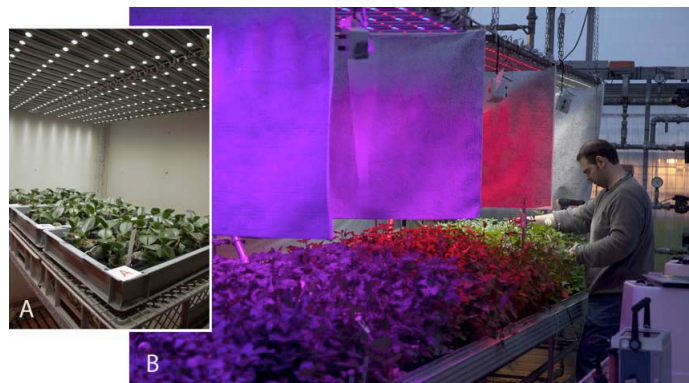
Figure 4.4: Philips' adjustable research modules with high efficiency LEDs: (A) white LEDs mounted in climate chamber (for which the research modules are designed) and (B) four modules used in a greenhouse (from left 40% blue in red, 20% blue in red, 100% red and white LEDs). In the climate chamber this setup of modules can be adjusted up to ca 300\mu\text{mol m}^{-2} \text{s}^{-1} . Note that the white treatment looks brighter to the eye than the red and blue combinations, despite that all four colours give identical PPFD. Photograph: Eva Rosenqvist.
