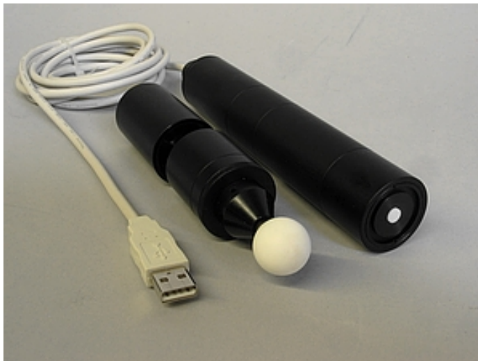
Figure 3.4: 'AMOUR' USB radiometers. Left: With a spherical diffuser for measuring fluence rate; right: with a planar cosine diffuser for measuring irradiance. Photograph © by Biospherical Instruments Inc.
