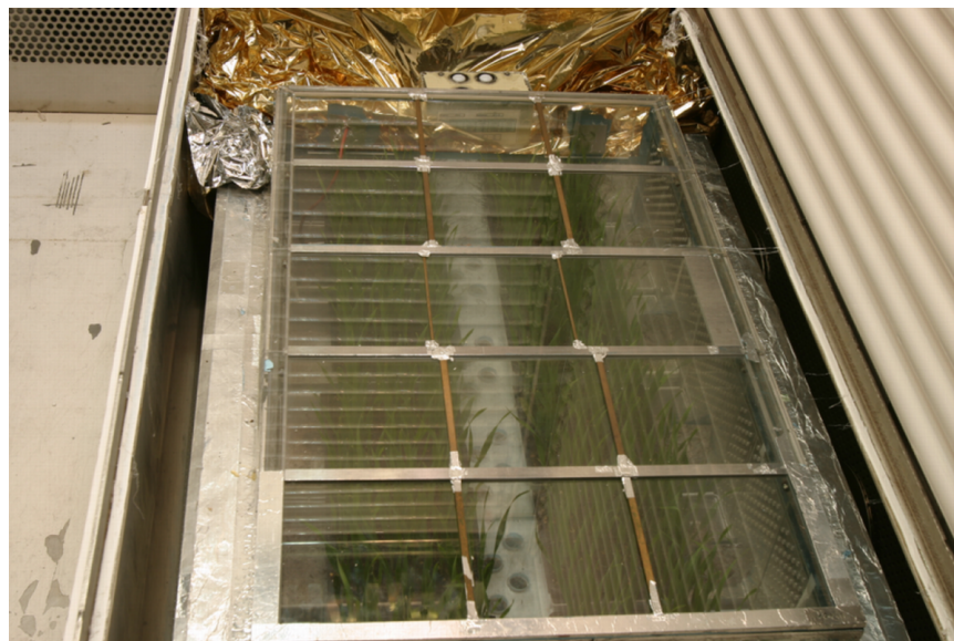
Figure 1.21: Special cuvette in the small sun simulator of the Helmholtz Zentrum München (see section 2.2.7 at page 48) covered by five coloured glass filter from Schott, Mainz, Germany, to simulate five different UV scenarios. The filters from top to bottom are WG295, WG305, WG320, WG335 as well as WG360. The resulting spectral irradiances in the UV range for one specific incoming radiation is shown in figure 1.20 in section 1.8.2 on page 24. Photograph: Andreas Albert.
