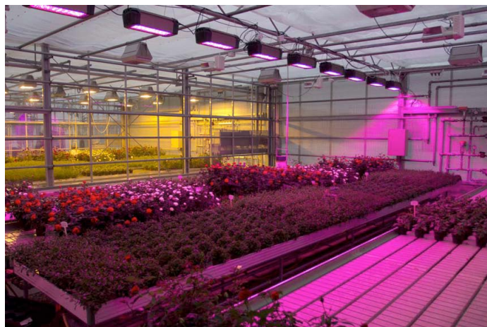
Figure 4.5: Top light LED lamps (Fionia Lighting, DK) tested for plant growth and energy consumption for light and greenhouse heating, in comparison with high pressure sodium lamps in the next greenhouse compartment. The setup gives supplemental PPFD of 120 \mu\text{mol m}^{-2} \text{s}^{-1} at a distance of 2.2 m from the bench, which is a level used for high light demanding species in production. Photograph: Carl-Otto Ottosen.
