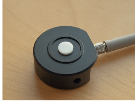
Figure 3.20: Bentham D7-H-SMA cosine diffuser. Photograph: Pedro J. Aphalo.
