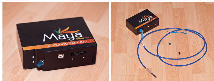
Figure 3.16: Left: Maya 2000 PRO spectrometer. Right: The same instrument connected to an optical fibre and a small cosine diffuser. Spectrometer and accessories from Ocean Optics. Photographs: Pedro J. Aphalo.
