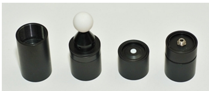
Figure 3.3: Different entrance optics used in USB radiometers of the ‘AMOUR’ series. From left to right: radiance, fluence rate (or scalar irradiance), irradiance and SMA connector. The SMA connector can be used to attach an optical fibre. Photograph © by Biospherical Instruments Inc.
