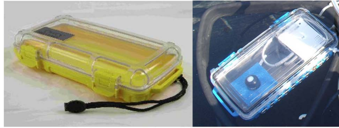
Figure 3.24: Hermetic water -proof housing without and with light sensors and data logger inside of the box. Photographs © EIC (Equipos, Instrumentación y Control).
