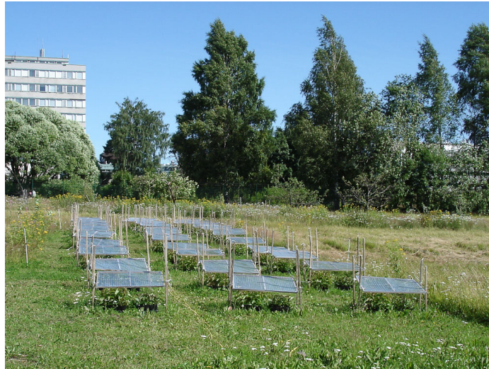
Figure 2.23: Filters in the field, mounted on wooden frames, and slightly tilted to avoid accumulation of rainwater. Viikki campus, University of Helsinki, Finland. Photograph: Pedro J. Aphalo.
