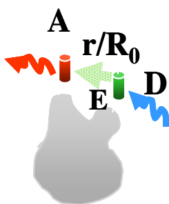
Fig. 1. Basic principle of FRET spectroscopy. A donor fluorophore (D) is excited and transfers this energy in a distance- and orientation-dependent manner ( r/R_0 ) to an acceptor molecule (A). The energy transfer between an excited donor to an acceptor occurs through non-radiative dipole-dipole coupling (E). This process is called "Förster resonance energy transfer".
