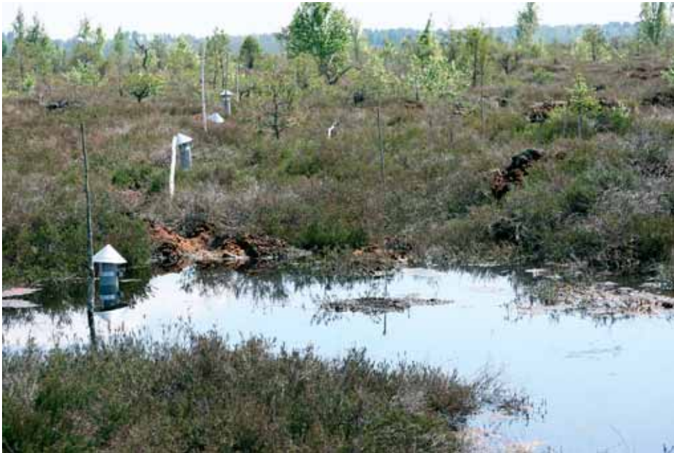
Figure 14. Water table monitoring wells and habitat monitoring relevés in Vasenieki Mire (Photo M. Pakalne).
