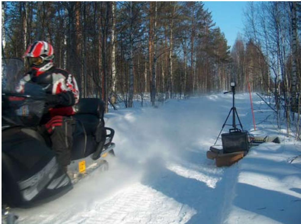
Figure 4. The speeds of individual snowmobiles were measured using radar.
