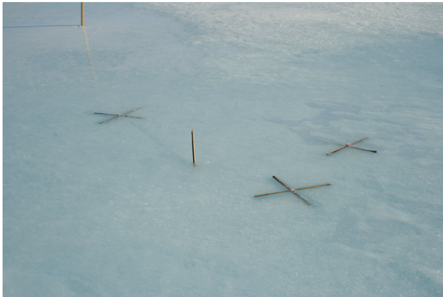
Figure 3.4: Light measurements inside ice. PAR sensors are hanging down from bamboo crosses for different depths.
