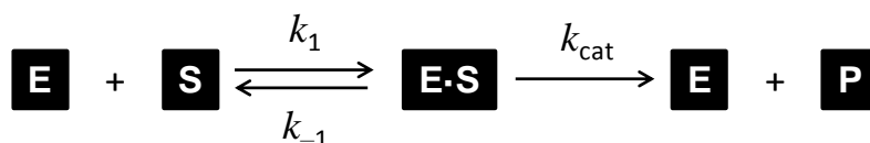
Figure 15. A simplified scheme of the enzyme reaction used to derive the Michaelis-Menten equation.
