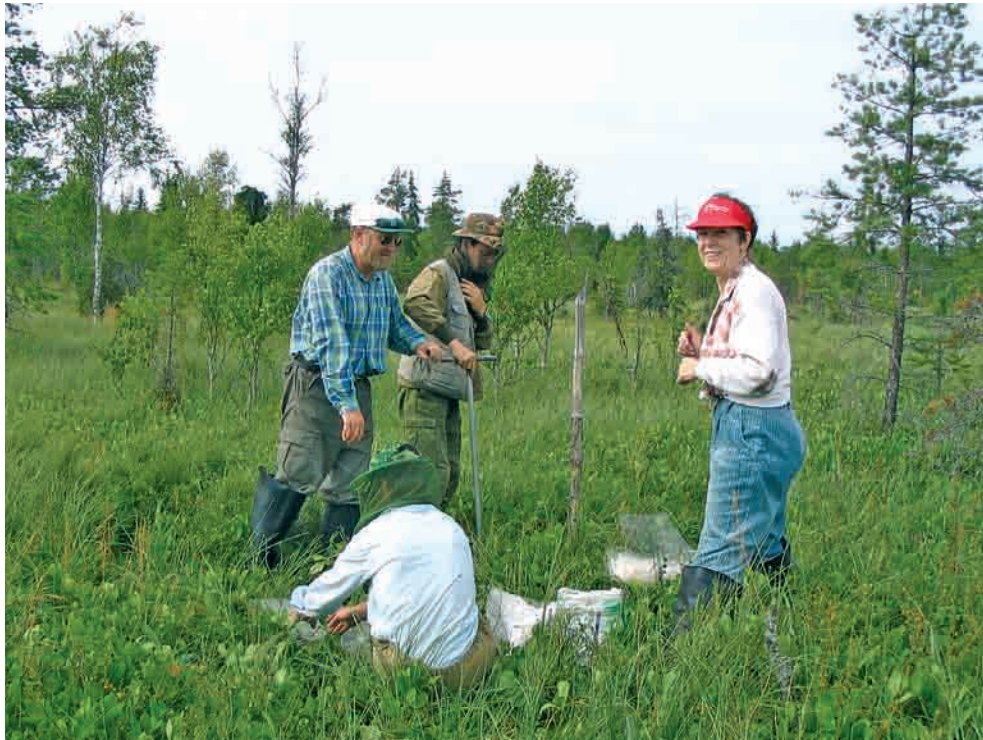
Fig. 36. Dr. Oleg Kuznetsov and the staff of the Mire Ecosystems Laboratory drilling a peat deposit to obtain samples for pollen and botanical analyses. Shown below are samples with (a) peat of varying botanical composition and (b) clay. Photo: G. Elina
