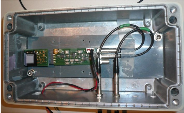
Fig. 5. Charge sensitive pre-Amplifier connected to a U3DTHIN and linear amplifier.
