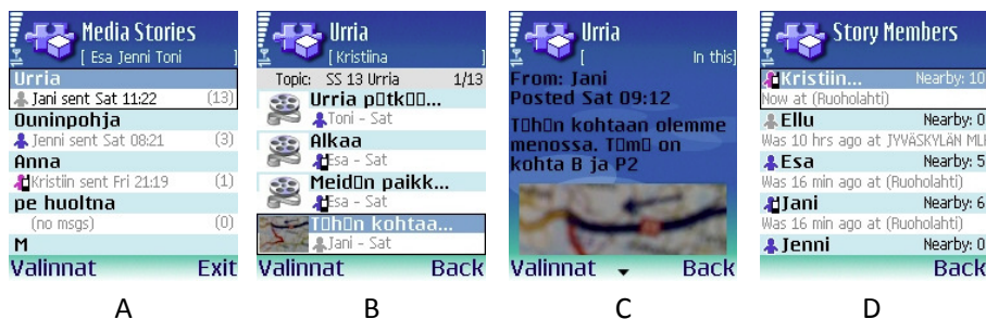
Figure 2.3: CoMedia's user interface. Unlike that of mGroup, the interface provides awareness information on all of its screens. The ticker box at the top of the screen informs about the other online users in the system (A), in the same media story (B), and in the same message (C). The users' online statuses were described by means of member icons and on a dedicated screen (D).
