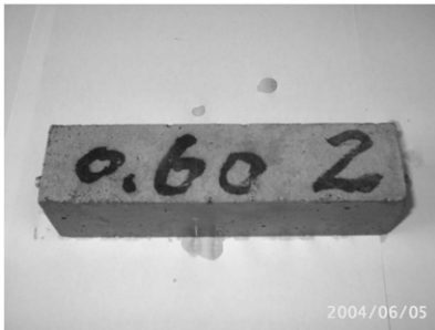
Fig. 1. Specimen of cement mortar with the w/c = 0.6 .
