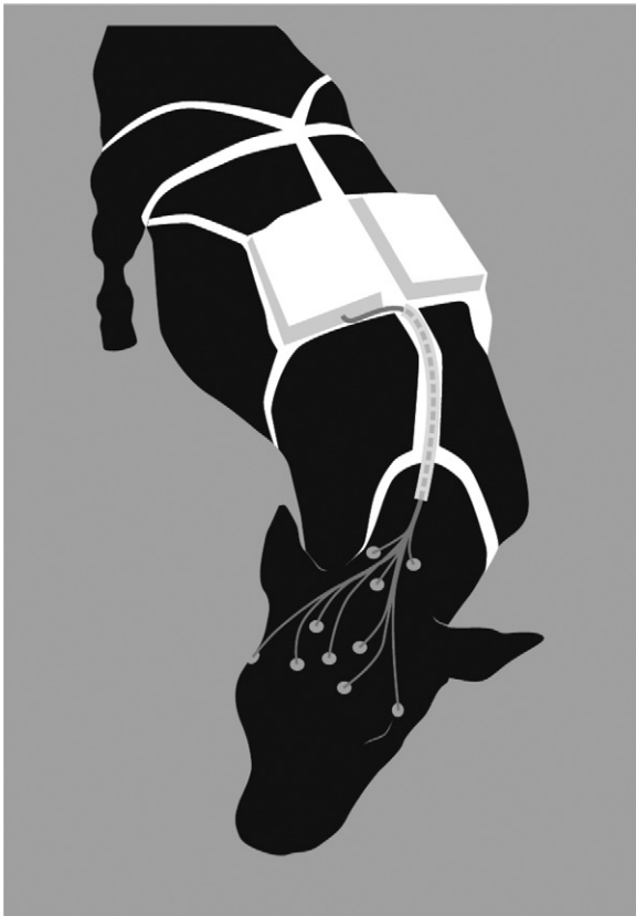
Fig. 1. Electrode placement and equipment for non-invasive EEG recordings in dairy cows. Snap-on electrode wires, which electrodes were connected to, were led to the device through a fabric tube. A counter weight is attached on the back of the cow, opposite the device.
