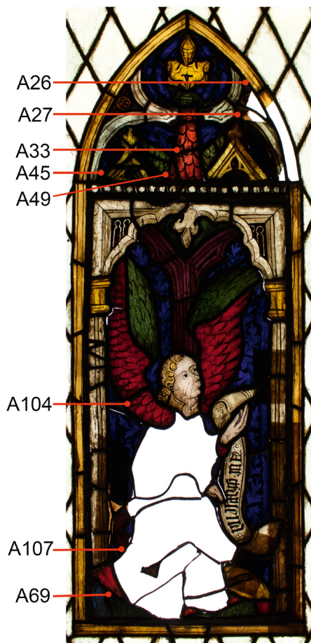
Fig. 2. Stained glass panel representing Annunciation Archangel Gabriel; Styria & Carinthia, about 1430; samples collected from different glasses for the analysis are indicated by a number and arrows.
