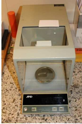
Figure 8. The A&D ER-180A (A&D Engineering, Inc., California, USA) electronic analytical balance was used to measure the mass loss of the Arabidopsis sample.
