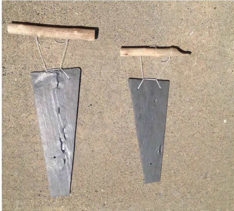
Figure A-3. Slate gongs constructed from 1/4 inch roofing slate
