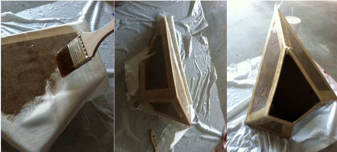
Figure 20. Fiberglass and Resin Application
