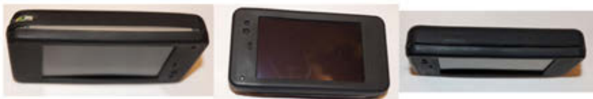
Figure 4: The device used in the experiments from outside with the silicon cover, as the users saw it. From left to right: the side of the phone with pressure the sensor, the front and the other side of the phone.
