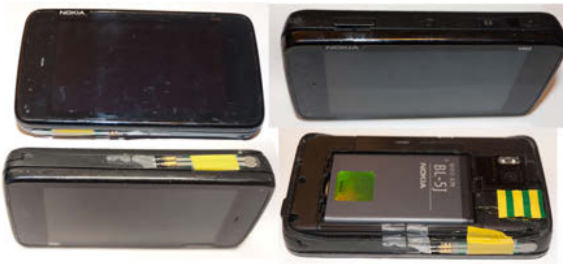
Figure 2: The device used in the tests from underneath the silicon covers. On the upper left corner the front of the phone, on the upper right corner the top of the phone with regular volume buttons and camera buttons, on the lower left corner the pressure measuring button and on the lower right corner the pressure device in the SD-cardslot.
