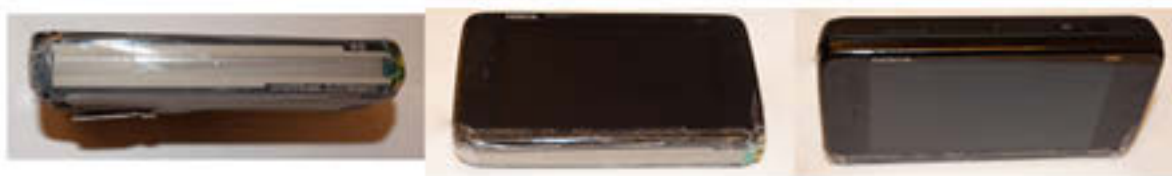
Figure 3: The device used in these experiments without the covers. From left to right: the side of the phone with the pressure sensor, the front and the other side of the phone, without the pressure sensor.
