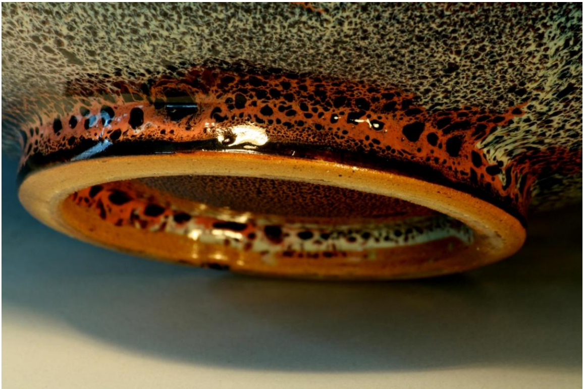
Figure 3- The sodium halo can be seen on the foot ring of this bowl. This is the foot for Figure 9. Notice the large spots around the foot and even underneath the bowl.
