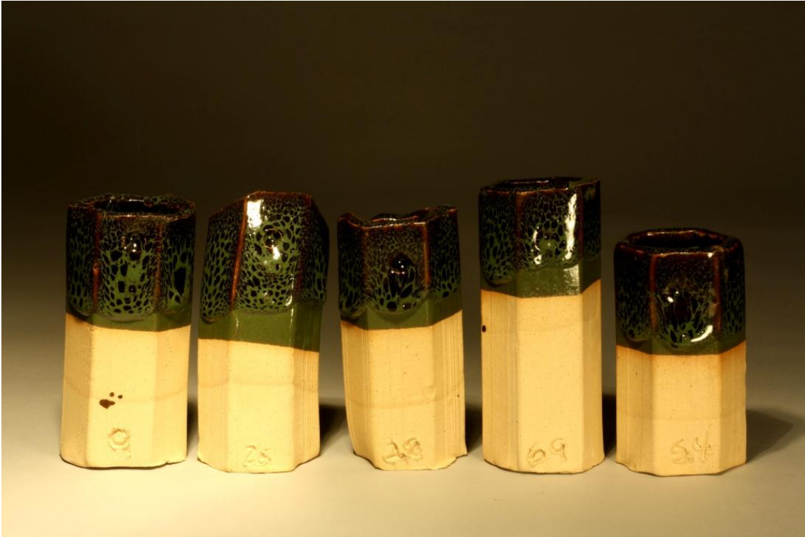
Figure 6- From left to right, one percent of dolomite was added. Notice the hanging glaze on the middle tile. The glaze is also smooth after one firing. The breaking of the glaze on the corners is very nice.
