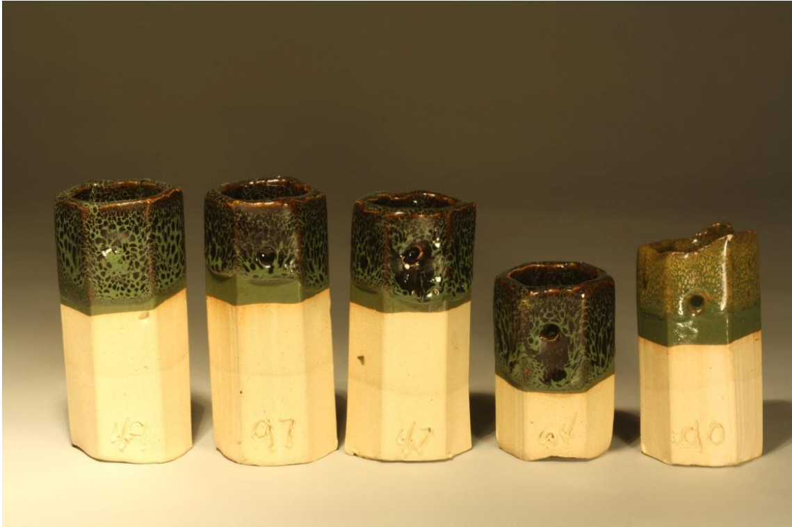
Figure 8- From left to right, one percent magnesium carbonate was added. Notice the yellow color of the far right tile. Five percent magnesium carbonate changes the color of the spot. The hanging glaze is not as noticeable.
