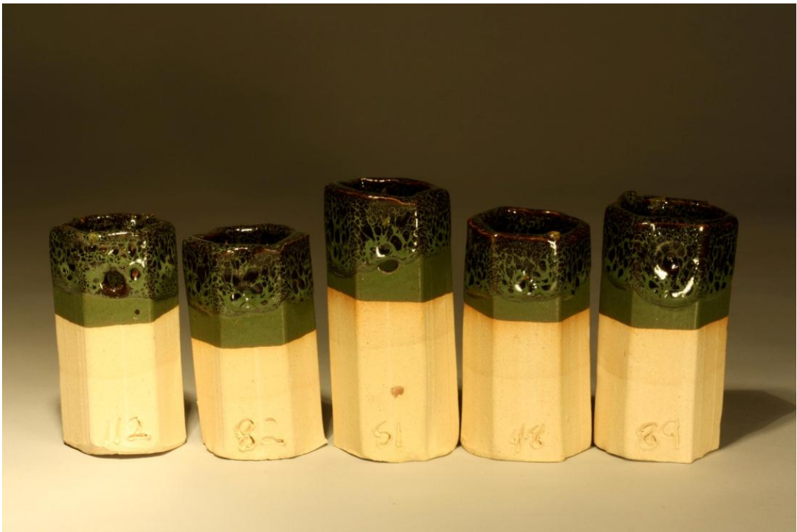
Figure 7- Five percent whiting was removed from the base. From left to right, one percent dolomite was added. Notice the pits and craters in the glaze. The hanging glaze is not even and not smooth.
