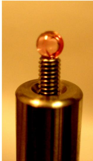
Figure 3.5: Actual Ti:Sapphire Lens
