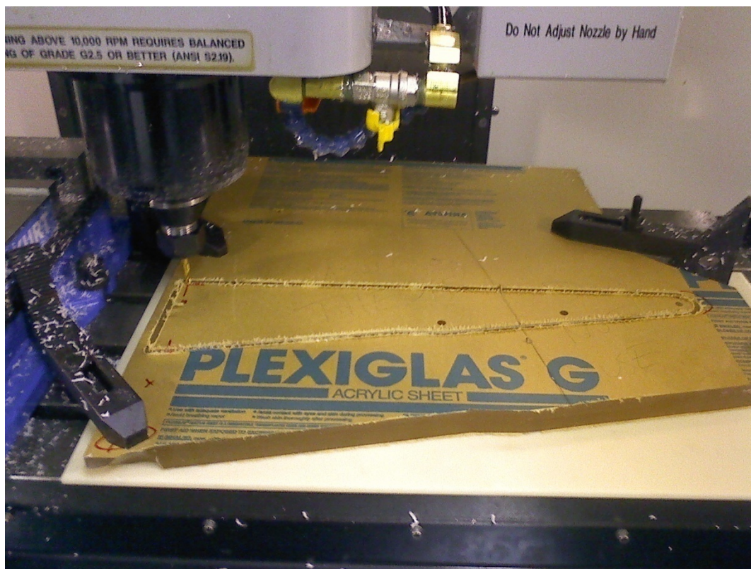
Figure 3.23: CNC subtractive machining performed to manufacture vertical supports used in final constructed device.
