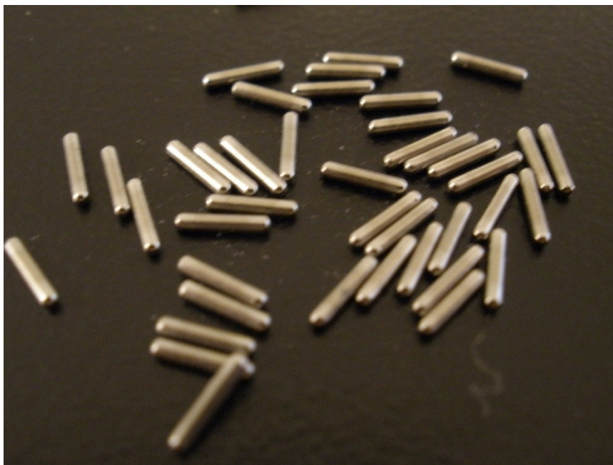
Figure 2.8: Photograph of typical brachytherapy source seeds used in permanent implant LDR procedures.
