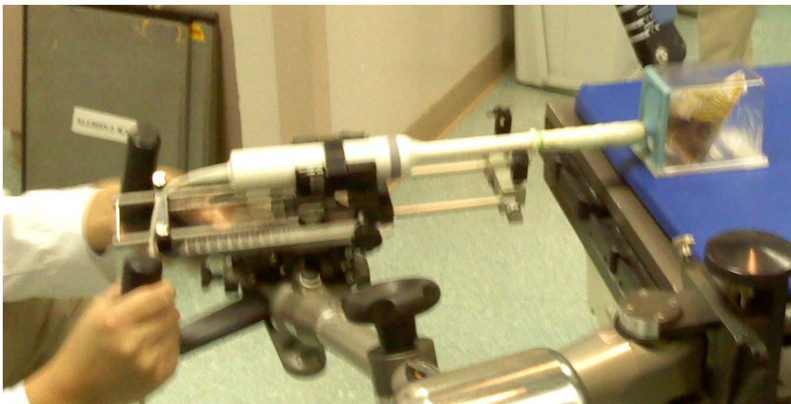
Figure 2.2: Example of transrectal ultrasound (TRUS) device used within the prostate brachytherapy process. SHANDS UF Hospital (2010). Photograph by J. Tyler Bennett (2010).
