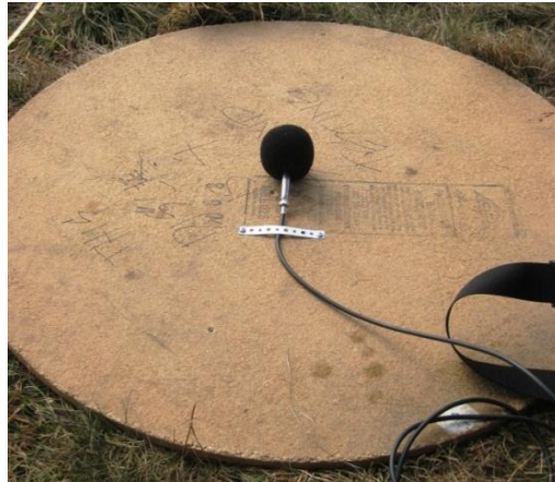
Figure 38. Picture of microphone mounted to circular plywood disc.
