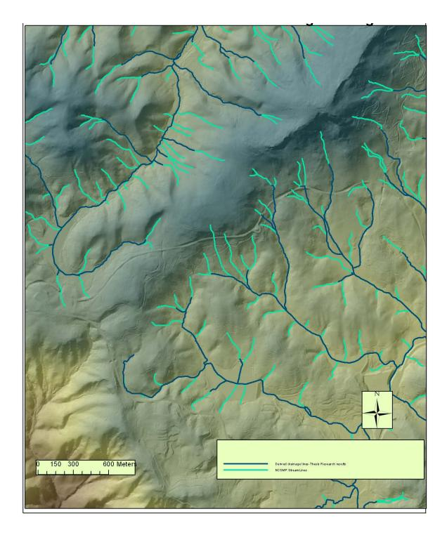
**Figure 15.** Derived drainage lines from this research (dark blue) with NCSMP drainage lines (light blue) displayed with 5 m DEM. Surface features such as gullies which contributed to generation of erroneous headwater segments of NCSMP are observable.
