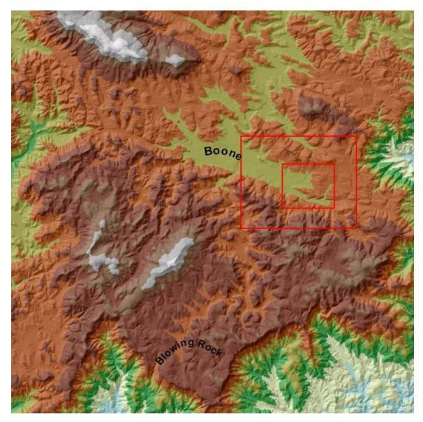
**Figure 4.** Terrain dataset of entire study area, including 25 bare earth LiDAR tiles from the NCSMP. Study area measures approximately 15,240 meters by 15,240 meters.
