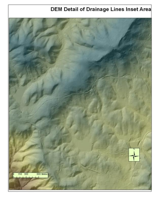
**Figure 13.** Five meter DEM of area near Blowing Rock generated from natural neighbors interpolation of terrain dataset derived from bare earth LiDAR. No hydrography features are displayed in this image. Surface and elevational features are clearly visible.
