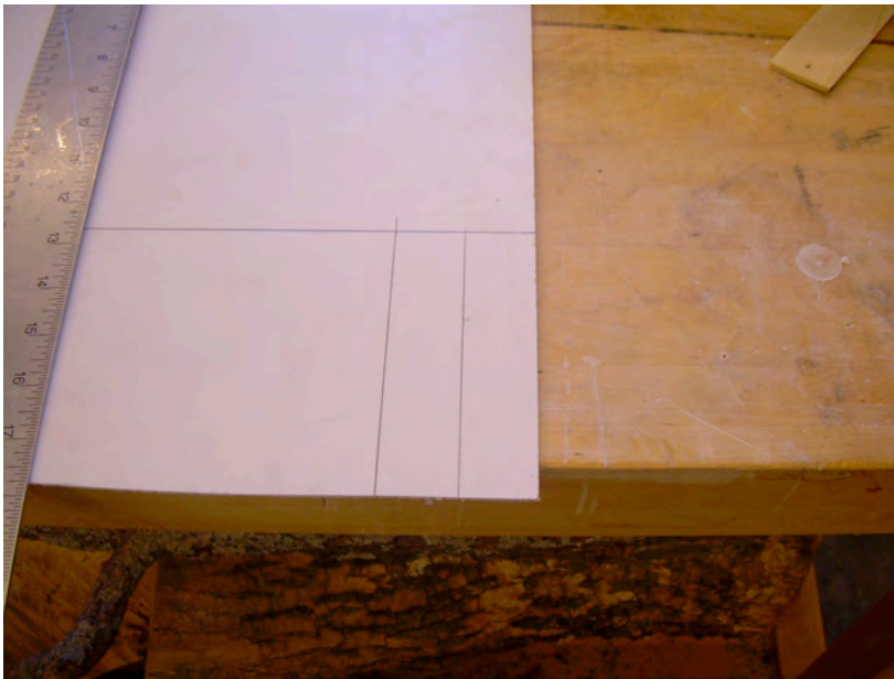
Figure 43: Measured sheet of polystyrene.
