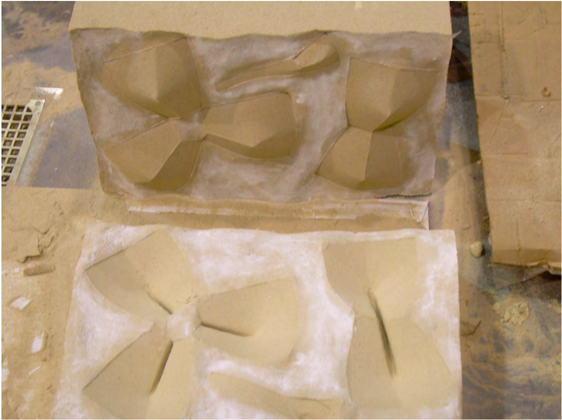
Figure 32: Chipboard models removed from bottom half of two-piece mold.
