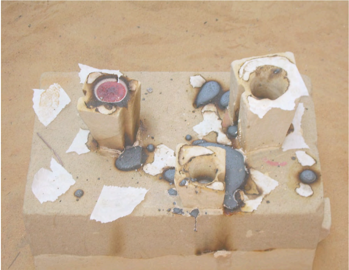
Figure 36: Excess of poured iron in the two-piece mold.
