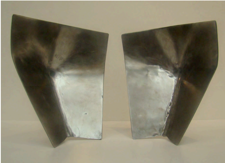
Figure 96: 7.5 x 7.5 inch 16 gauge carbon steel food scoops. (Note: Food scoops were sand blasted and polished to simulate stainless steel.)
