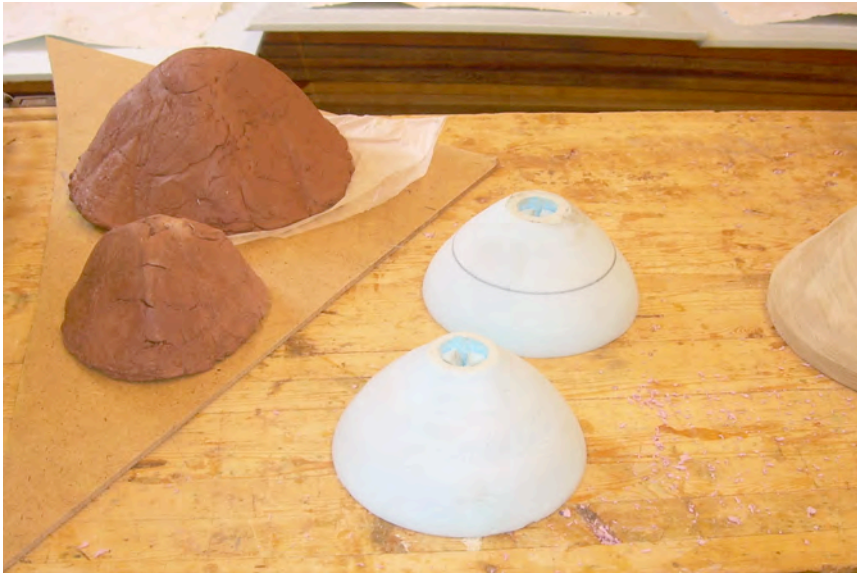
Figure 79: Clay negative of interior of stainless steel nesting bowl.
