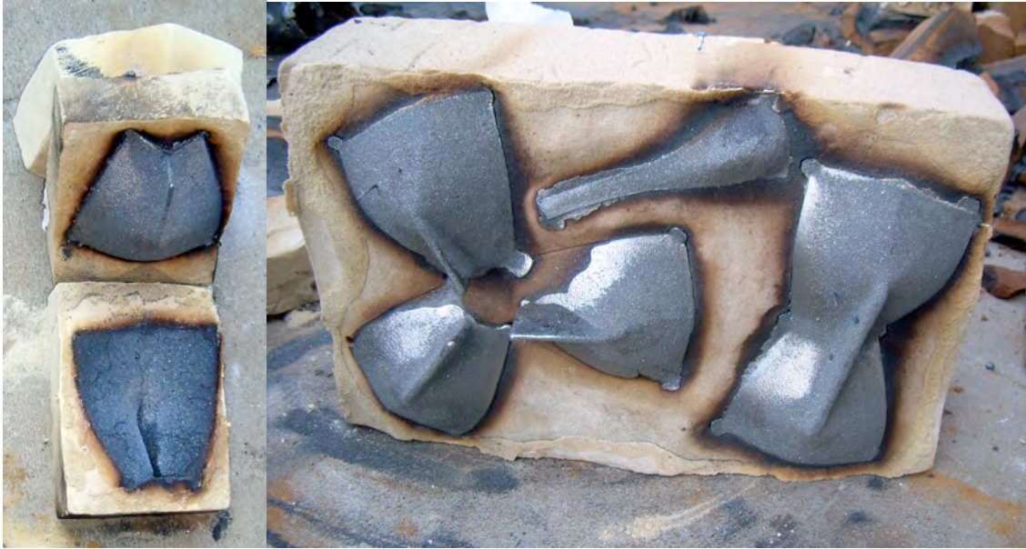
Figure 37: Solidified cast iron food scoop, serving tray and spoon. (Note: These cast pieces are attached to the top half of the two-piece mold due to the metal sprues and vents that formed during the metal pouring).
