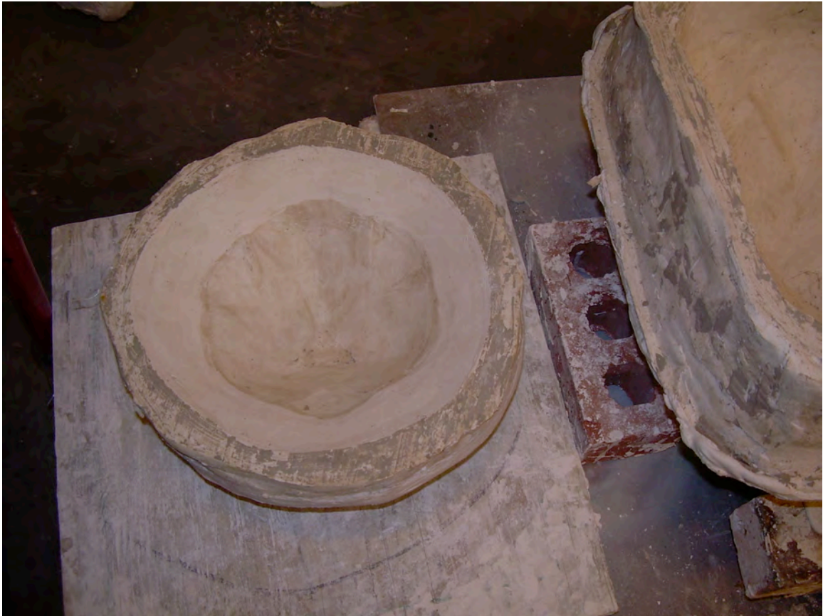
Figure 90: Clay removed from plaster mold.
