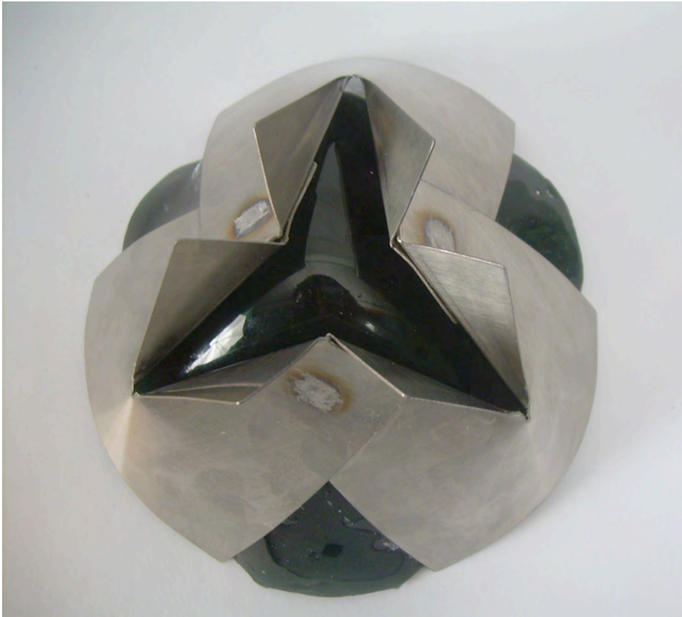
Figure 139: Bottom of slumped glass bowl. (Contoured to fit stainless steel serving vessel)
