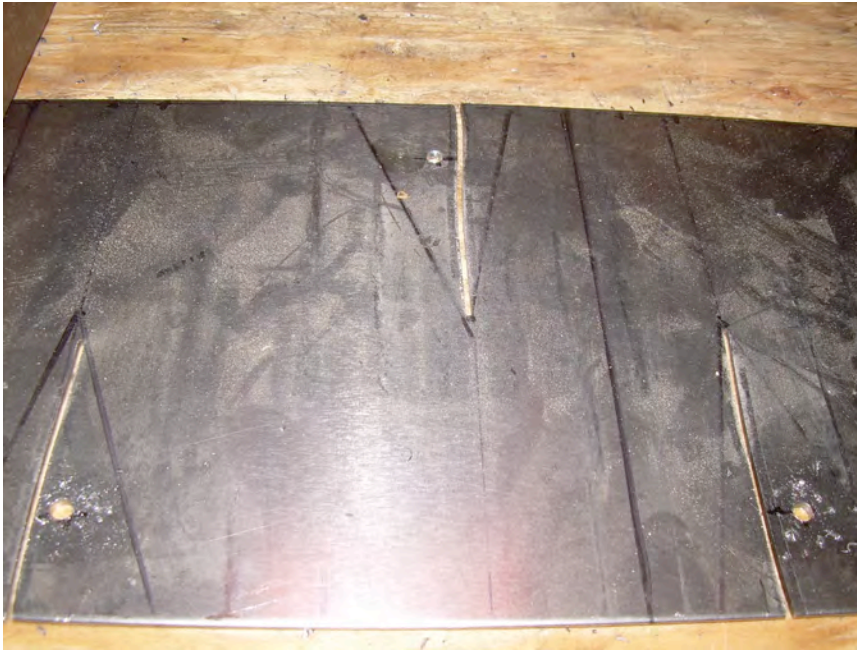
Figure 107: Slits of individual serving dishes cut with jigsaw.
