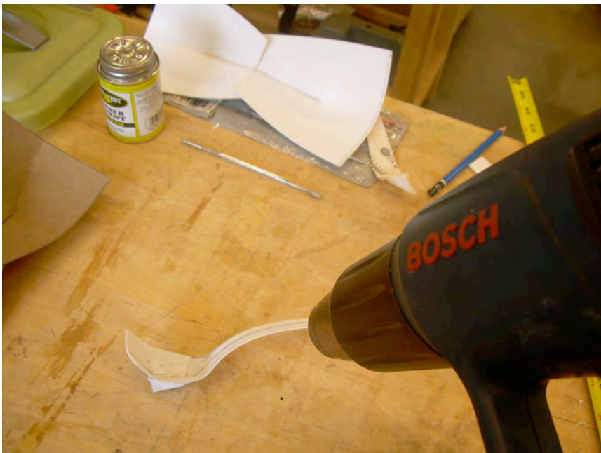
Figure 48: Polystyrene spoon handle heated with a heat gun.
