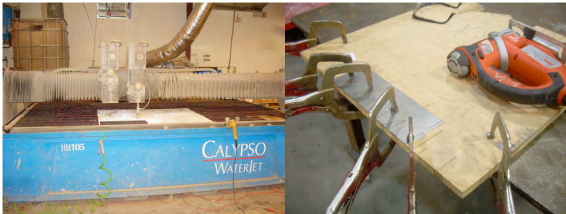
Figure 64: Left side: cutting sheet metal with an industrial water jet cutter. Right side: cutting the sheet metal with a jigsaw.
