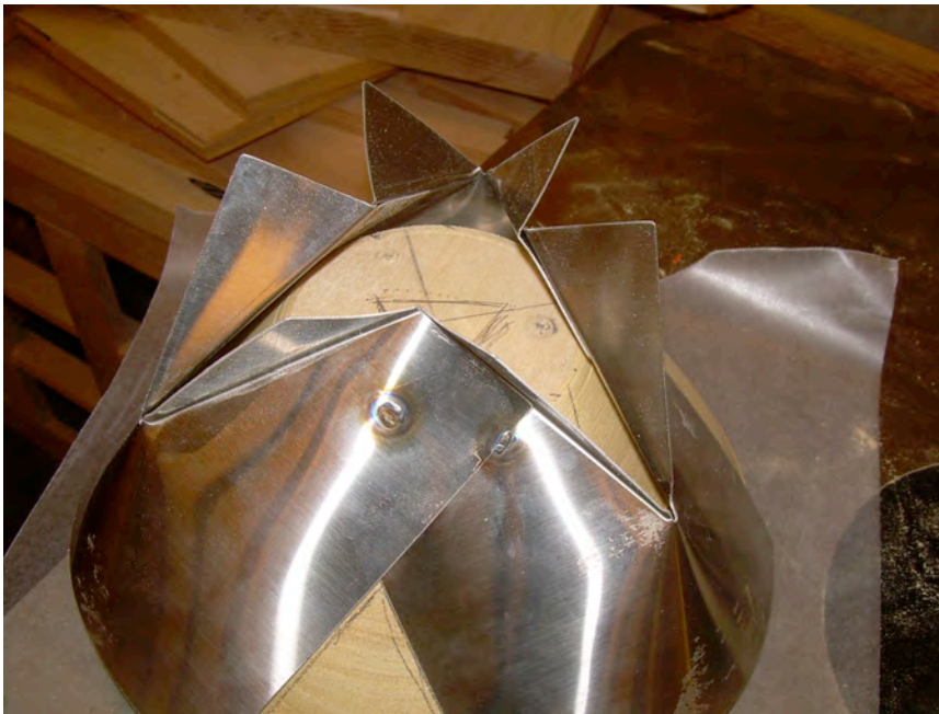
Figure 80: Measuring exterior of the bowl with the nesting bowl.
