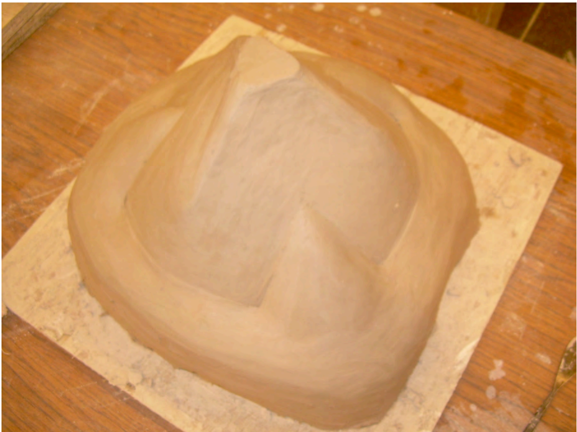
Figure 85: Clay negative of 9 x 9 x 9 inch nesting bowl interior. (Released from stainless steel nesting bowl and turned upside down)
