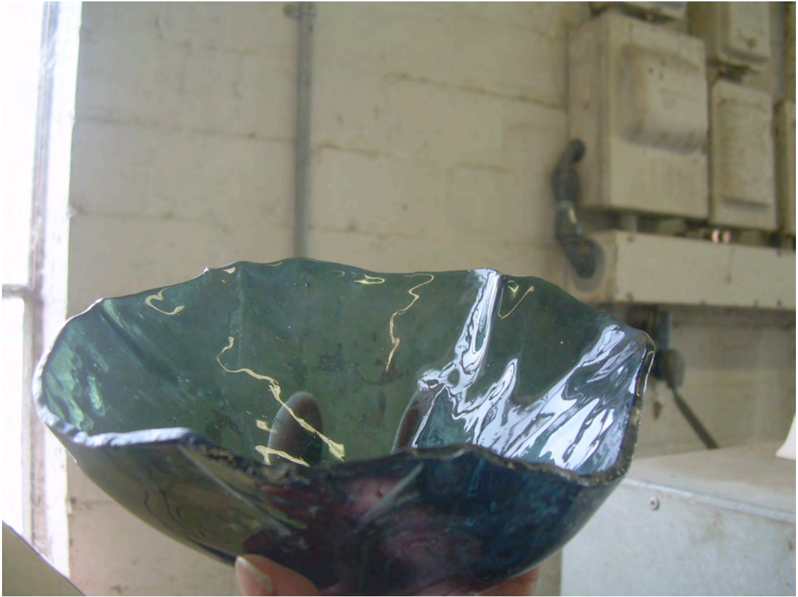
Figure 95: Slumped olive green glass bowl for 4 x 4 x 4 inch stainless steel bowl
