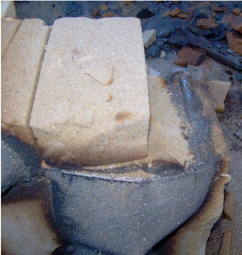
Figure 38: Sections of sand block chiseled away from serving tray vents.
