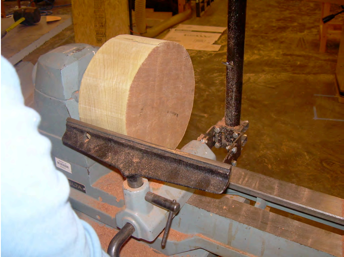
Figure 75: Poplar wood block attached to lathe.
