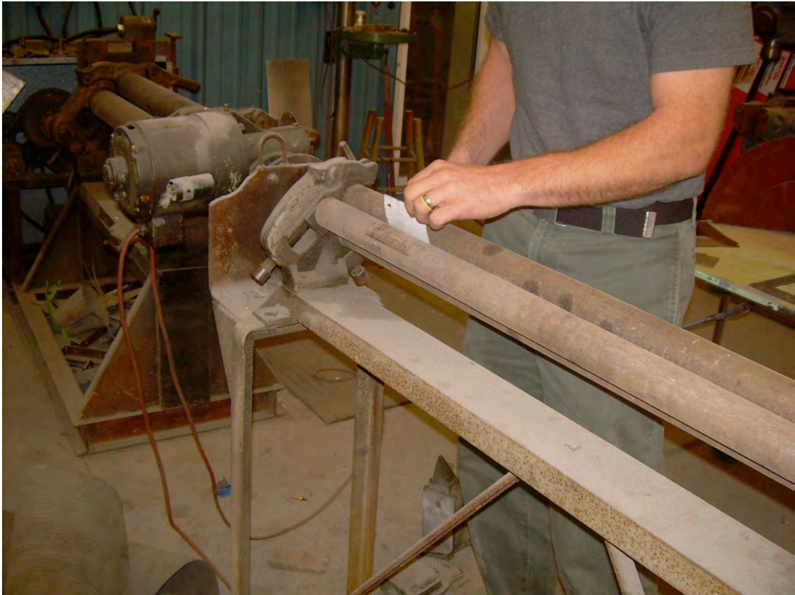
Figure 68: Curving the sheet metal with an electric roller.
