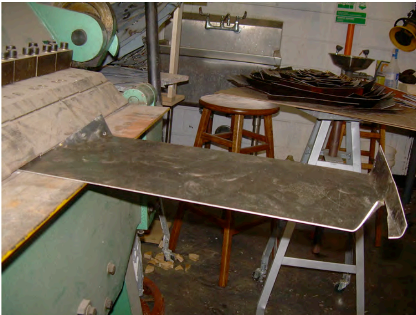
Figure 110: Cold bending with industrial brake.
