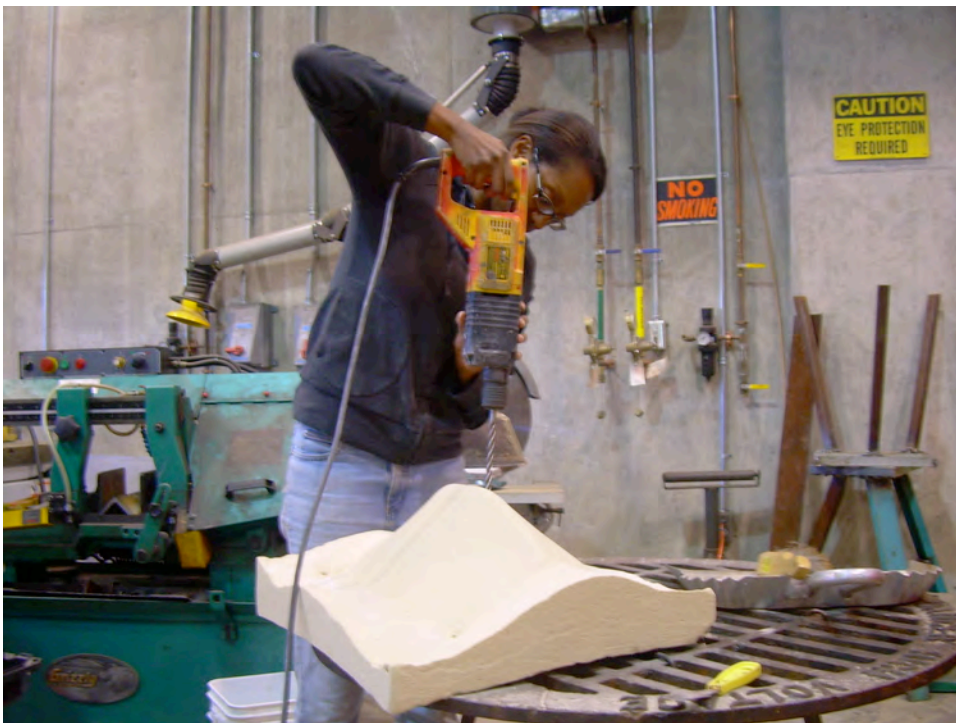
Figure 34: Drilling holes into the top half of the sand block using a hammer drill.
