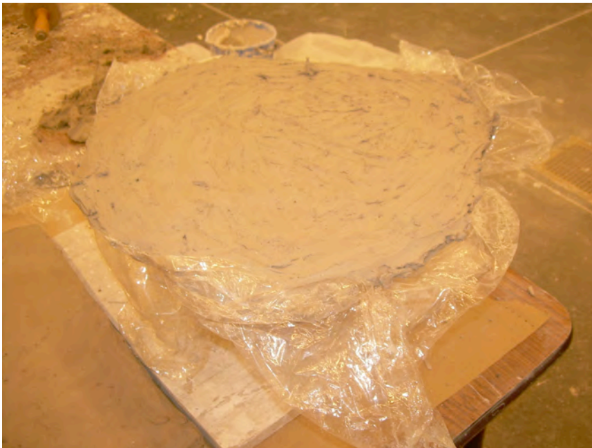
Figure 84: Top view of stainless steel nesting bowl filled with clay. Note: This was prior to turning it over onto the wooden board.
