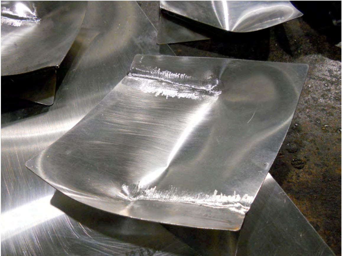
Figure 149: Extra water-jet sheets rolled through foundry roller. (Welded for individual serving dishes)
