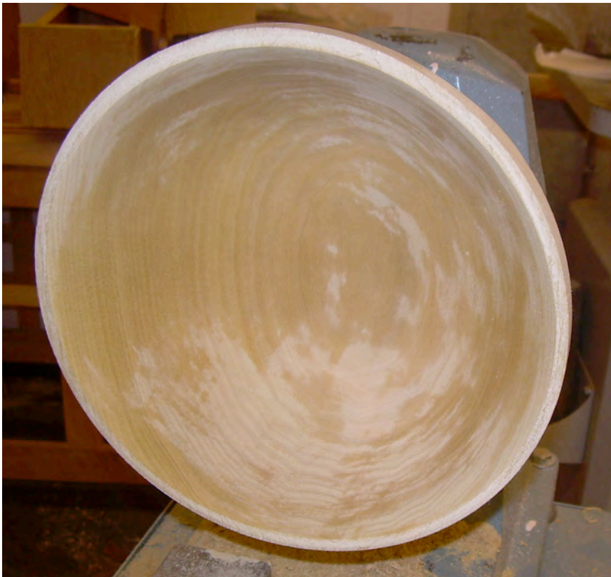
Figure 81: Wet sanding poplar bowl on the lathe.
