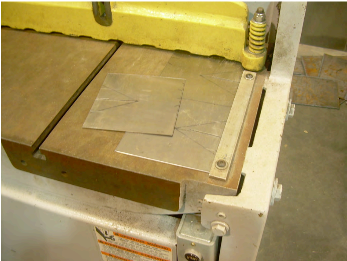
Figure 19: Cutting sheet metal with electric shear.
