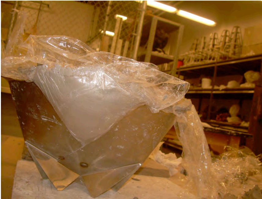
Figure 83: Clay pressed into the 9 x 9 x 9 stainless steel nesting bowl.
