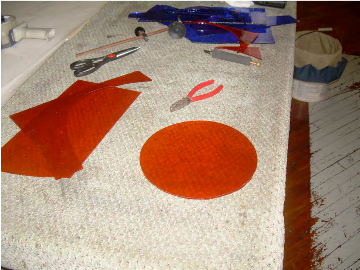
Figure 92: Cut glass sheets in the appropriate diameter.
