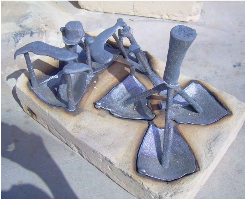
Figure 39: Cast iron serving trays and spoon with metal sprues and vents attached.
