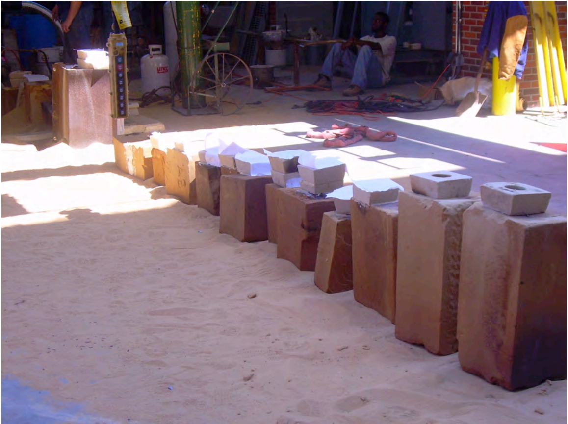
Figure 26: 2010 Spring, Sand Block Molds lined up for Metal Pouring.
