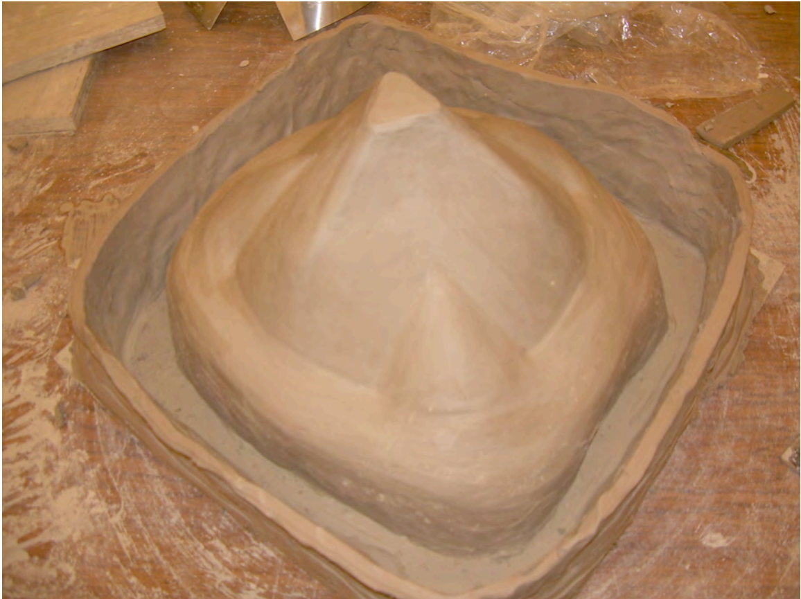
Figure 86: Clay slip and clay wall applied to the border of the clay negative.
