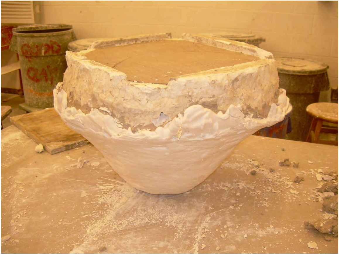
Figure 89: Plaster mold removed from base and turned over with clay.
