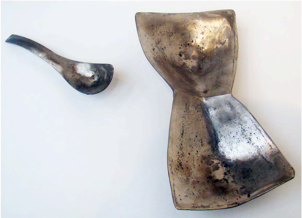
Figure 105: Cast Iron Prototype of 4.5 x 9 inch Dual Serving Tray and Spoon
