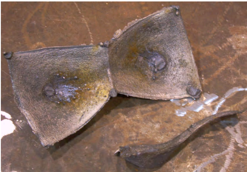
Figure 40: Cast iron serving tray and spoon with sprues and vents removed.
