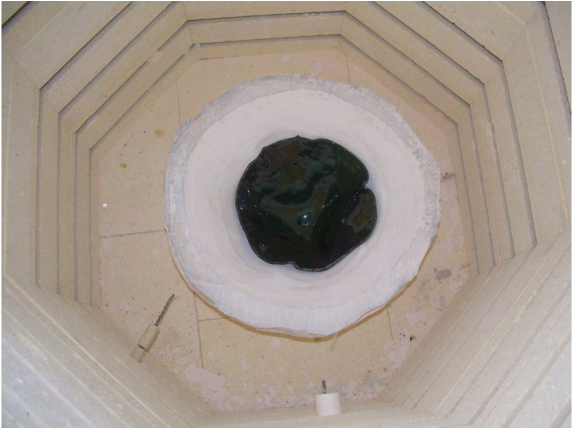
Figure 94: Glass slumped inside of plaster mold after it's fired inside the kiln.
