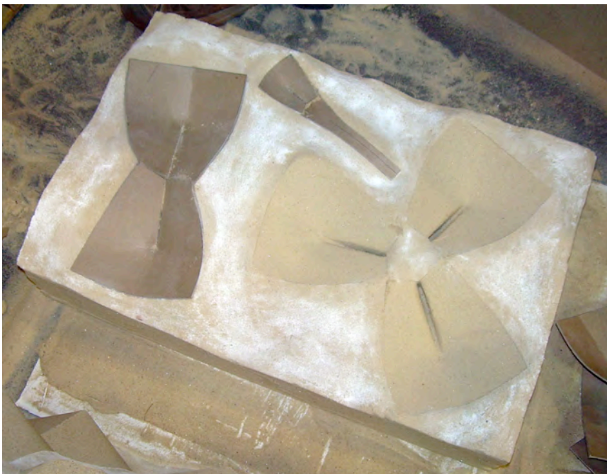
Figure 31: Chipboard models of serving tray and spoon. (Nested in the bottom half of the sand block).
