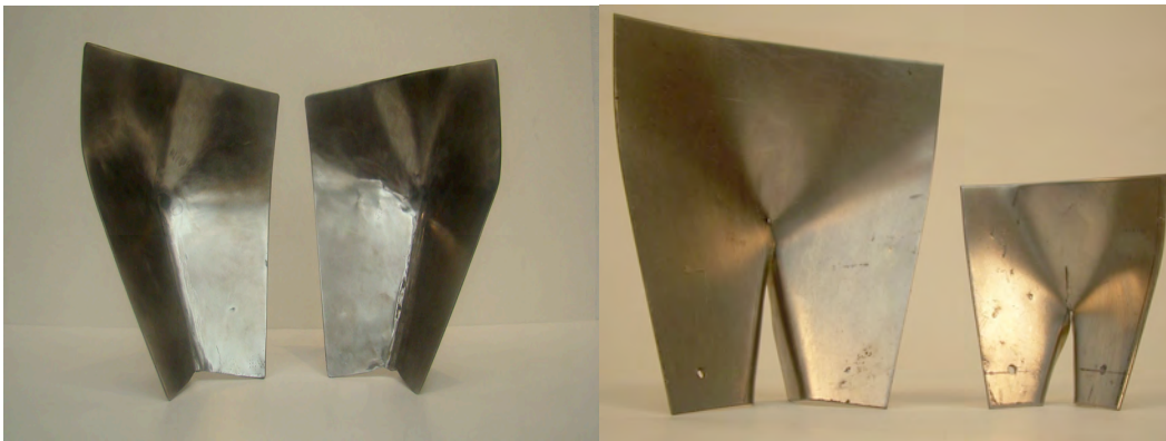
Figure 115: Welded slits versus open slits of the scoop form.
