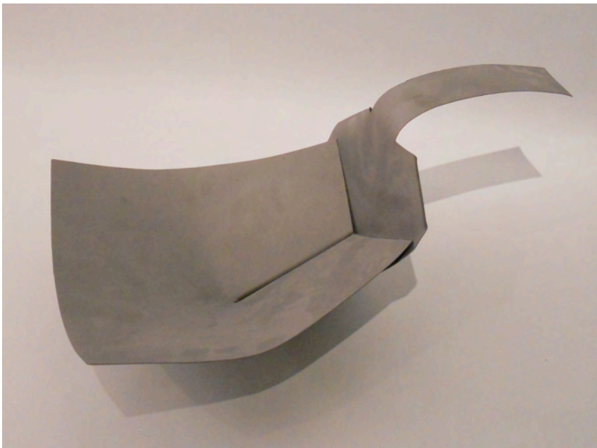
Figure 97: 12 x 12 inch 16 gauge carbon steel cooking utensil. (Note: Cooking utensil was sand blasted and polished to simulate stainless steel.)
