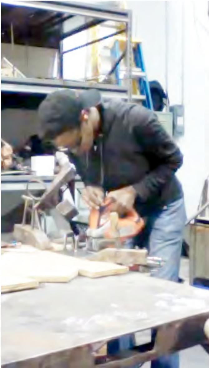
Figure 20: Cutting sheet metal clamped to wood with a jigsaw.
