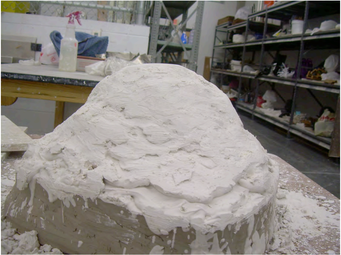
Figure 88: Plaster mold applied to clay negative.
