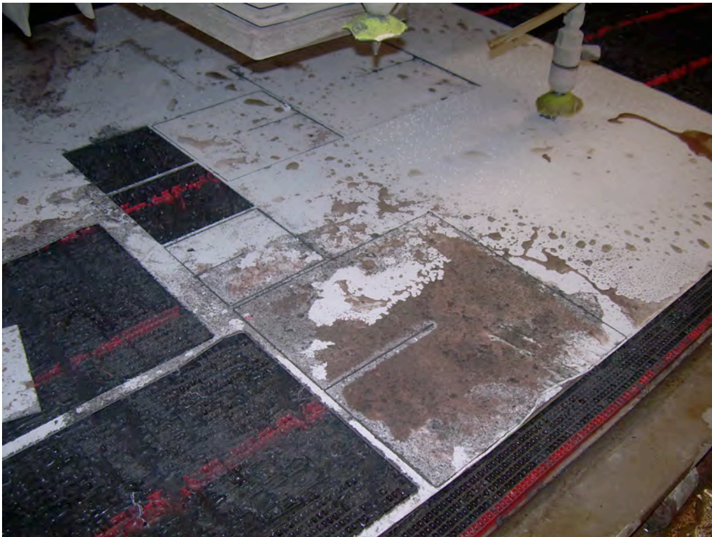
Figure 66: Water jet cutting sheet metal. (9 x 9 x 9, 6 x 6 x 6, and 4 x 4 x 4 inch layouts)
