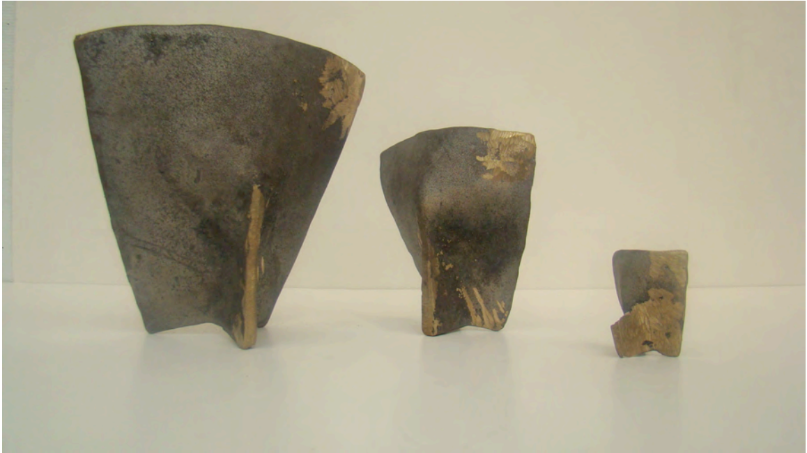
Figure 27: Cast Bronze models of scoop with removed sprues and vents.
