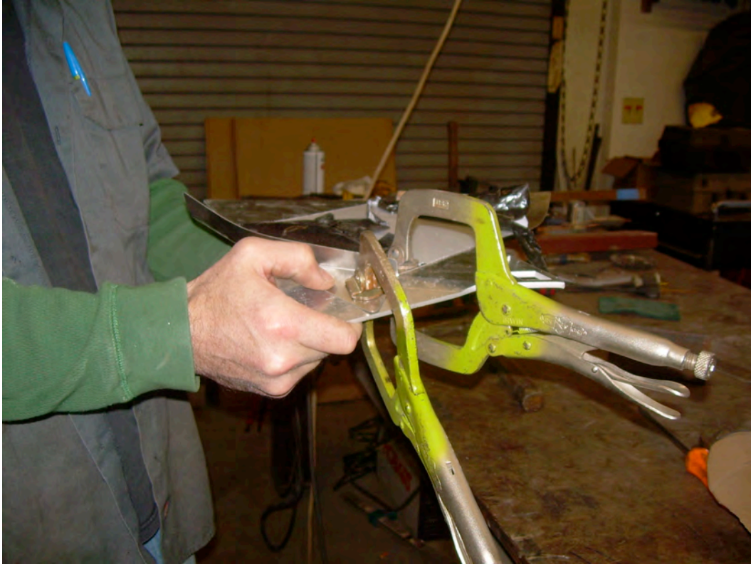
Figure 70: Welded sheet metal clamped to aluminum.
