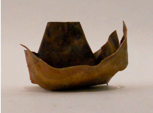
Figure 6: Copper Heated with a torch and bent.
