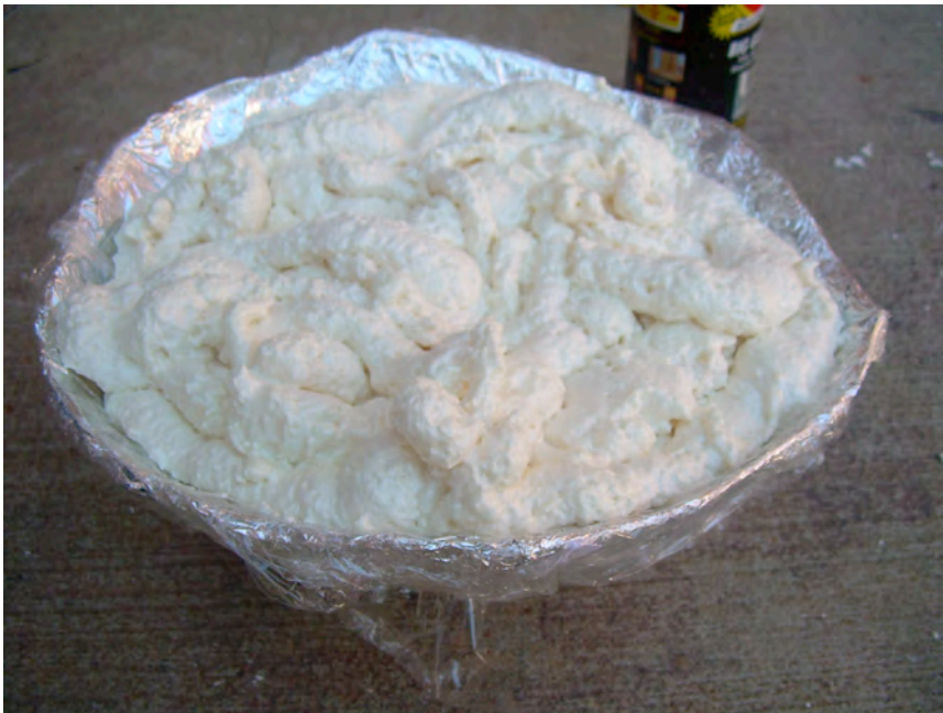
Figure 78: Insulated foam sprayed into a stainless steel nesting bowl. Note: The stainless steel bowl was covered in aluminum and saran wrap in attempt to preserve the stainless steel finish.
