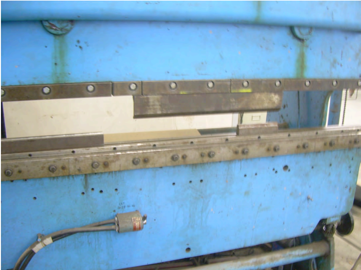
Figure 69: Breaking the sheet metal with an industrial brake.
