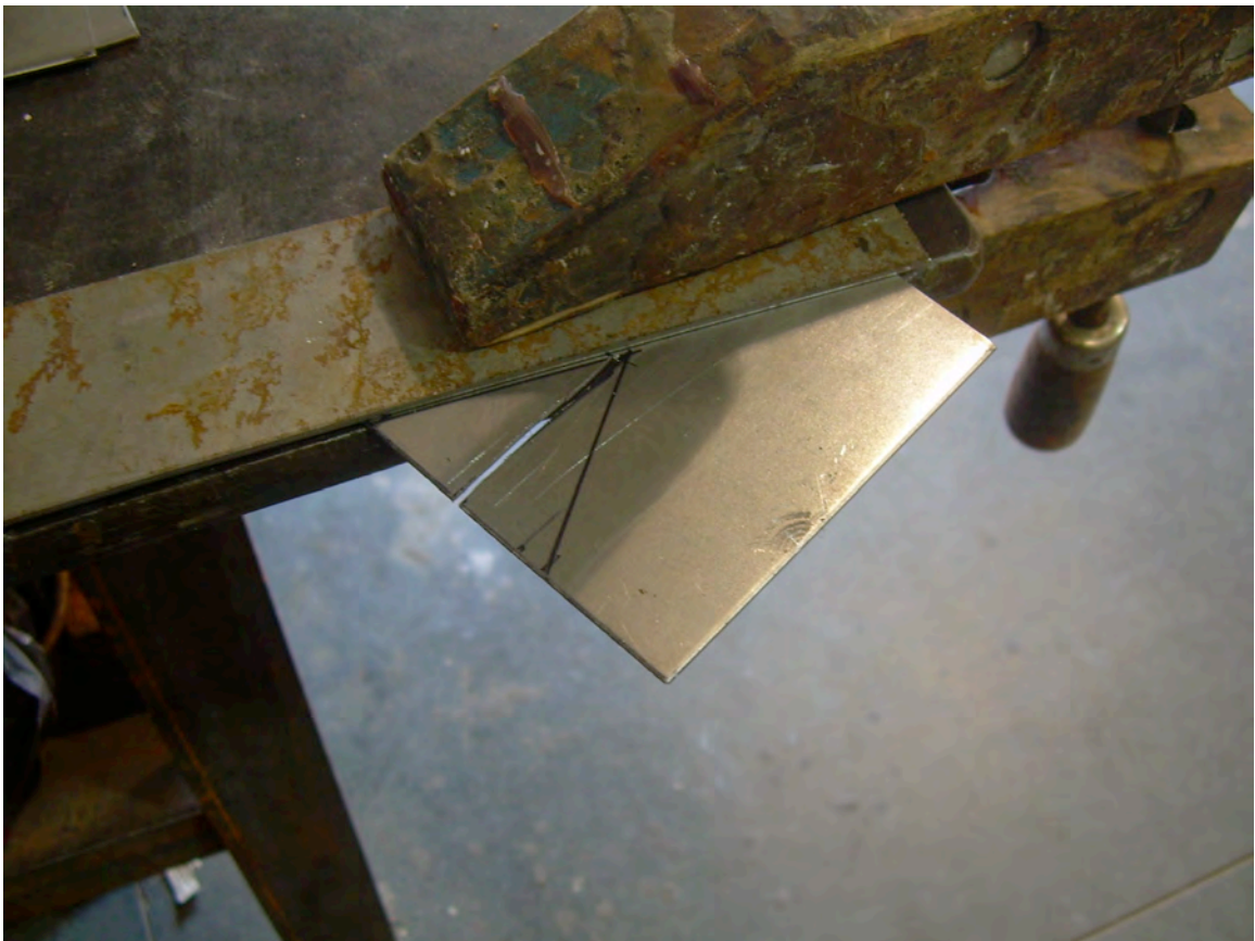
Figure 21:Clamping and bending sheet metal by hand.
