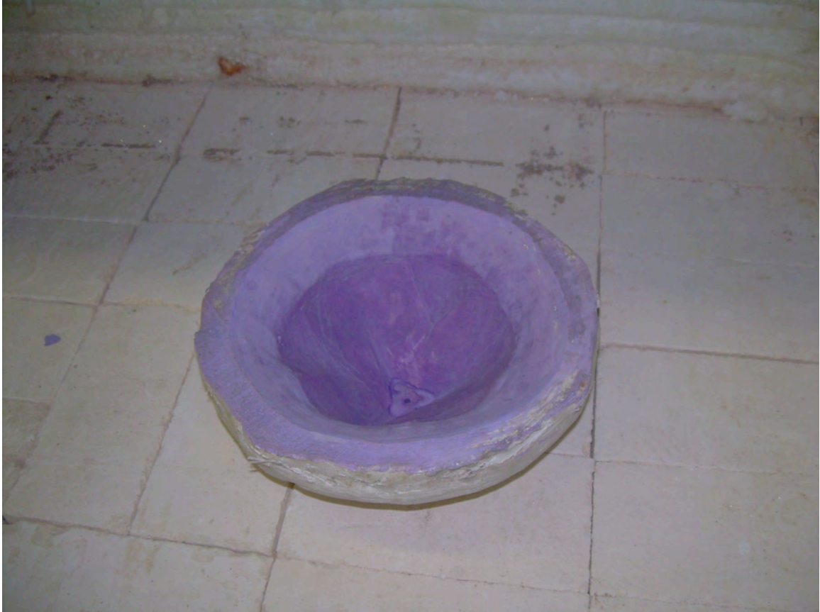
Figure 93: Interior of plaster mold coated with a primer. Primer was used to prevent the mold from cracking during the firing process.
