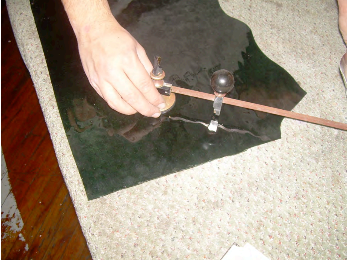
Figure 91: Cutting selected glass sheets to the appropriate diameter.
