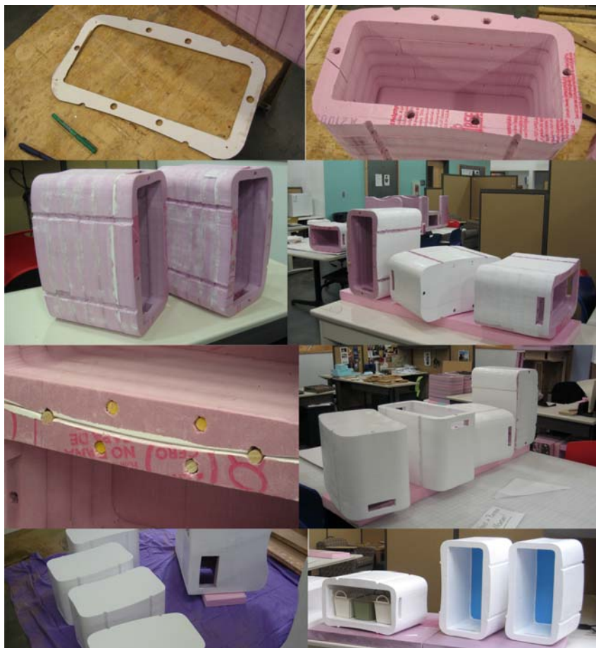
Figure 4.23. Construction Process of Final Small Foam Prototypes
