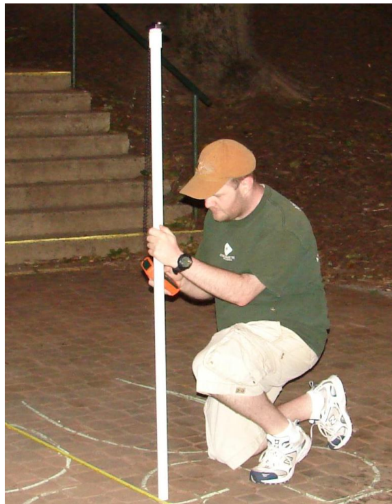
Figure 3. Diagram of Light Sampling Method and Testing Lux Values at 12.5 Feet from Lamppost Center.
