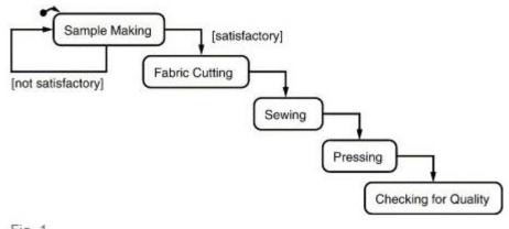
Fig. 1. A workflow in a simple garment factory.
