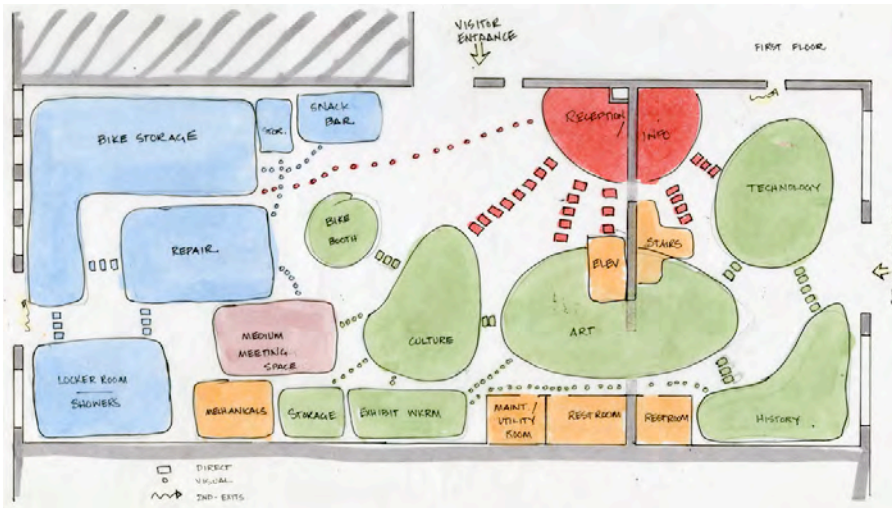
Figure 9. Bubble diagram of the first floor, used to determine adjacencies and circulation.
