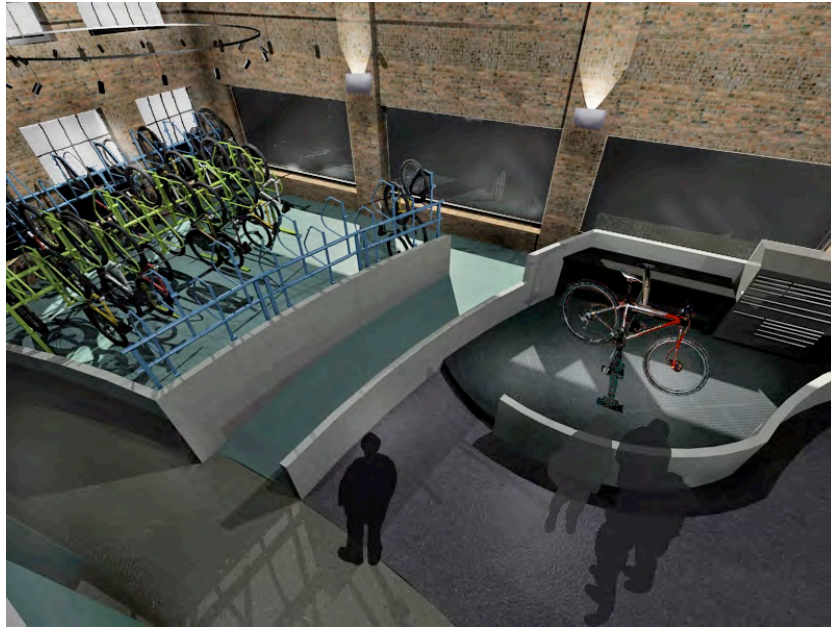
Figure 30. Birdseye view of the elevated bicycle storage and repair stand. The storage area, elevated two feet above floor level, accommodates 54 bicycles and operates as display space.
