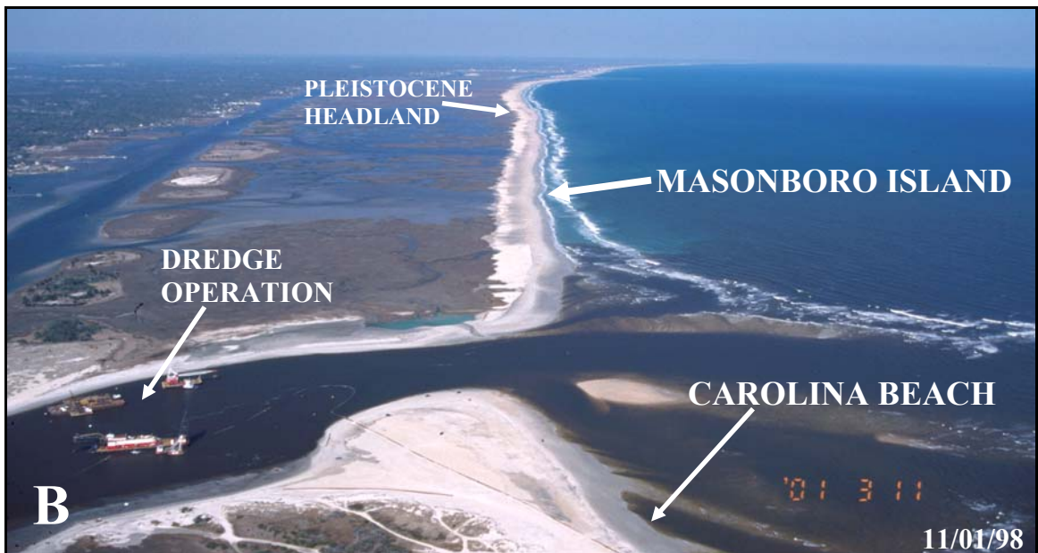
Figure 3. (A) Masonboro Inlet – the north jetty was completed in 1966 and the south jetty was completed in 1981. Note the impoundment of sand comprising the fillet adjacent to the south jetty. (B) Carolina Beach Inlet – this inlet was artificially opened in 1952 and must be repeatedly dredged to prevent closure. Photographs courtesy of William J. Cleary.
