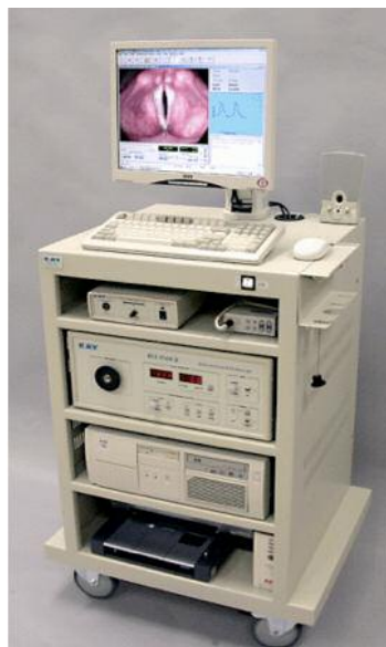
Figure 3. KayPentax LVES Workstation Showing Normal Vocal Folds on Screen. Digital Video Stroboscopy System, Model 9295 (used by permission)
