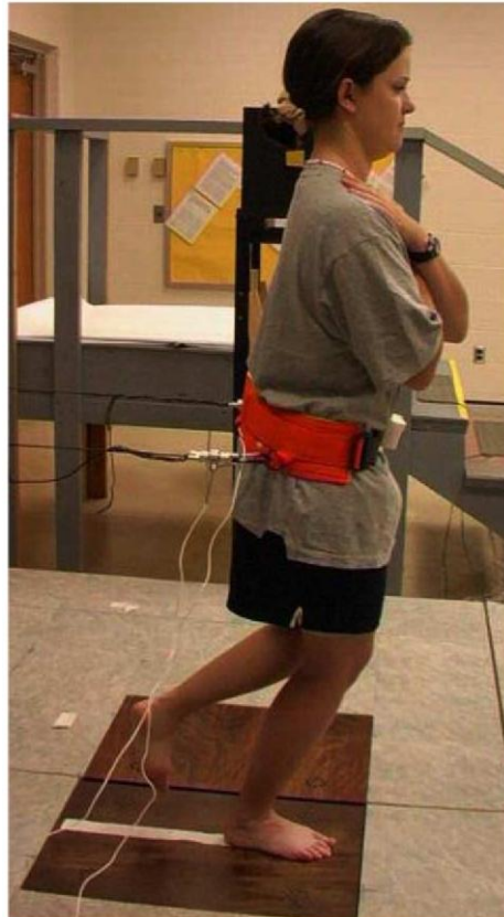
Fig. 1. Initial positioning — kevlar release cables attached to belt via load cells.
