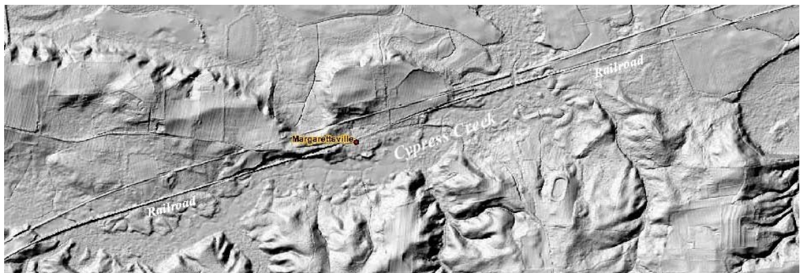
Figure 2. The route of the Portsmouth & Roanoke Rail Road entered North Carolina after crossing the Meherrin River. It followed the west bank of Cypress Creek until the bend past Margarettsville. It immediately begins an ascent to the “summit” at 144 feet.
