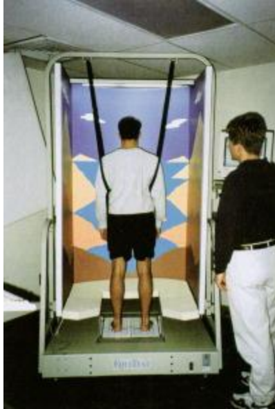
Figure 1-The NeuroCom Smart Balance Master (NeuroCom International Inc., Clackamas, OR) allows for sensory organization testing (SOT) using a dual force plate system. Both the support surface and visual surround tilt (sway referencing) to alter sensory conditions.
