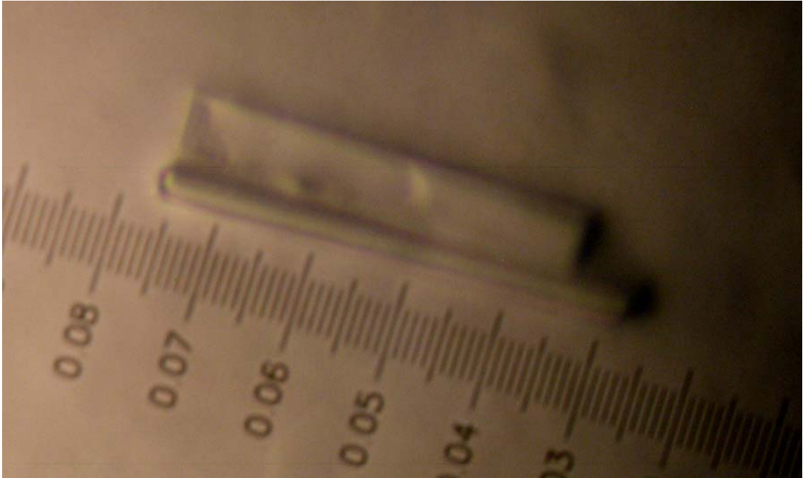
Figure 39. Picture of a crystallization drop showing a single crystal >0.2 mm in size.
