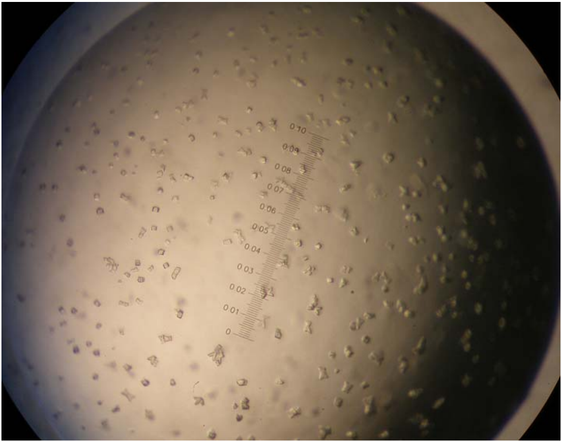
Figure 36. Picture of a crystallization drop showing crystals which are <0.2 mm and scattered throughout the drop.
