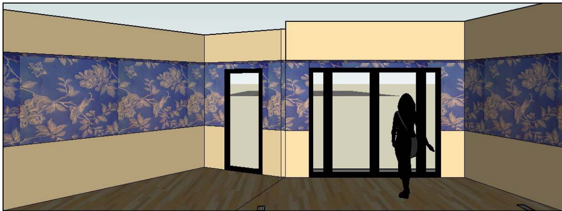
Figure 5.10: Exhibit space with fabric datum line 3 feet above the finished floor and 2 feet high
