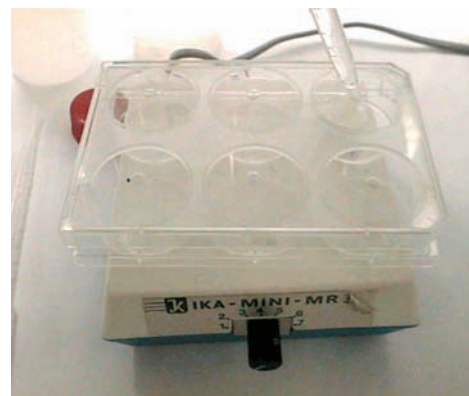
Figure 4. Green chemistry approach. A plastic microscale template used as a calorimeter.
