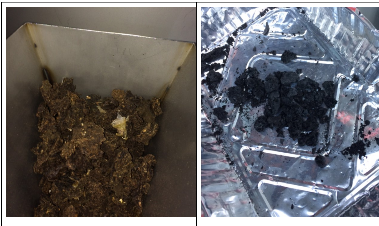
Figure 10 Dried human feces and resulting biochar after (mild) pyrolysis at 300°C for 20 min.
