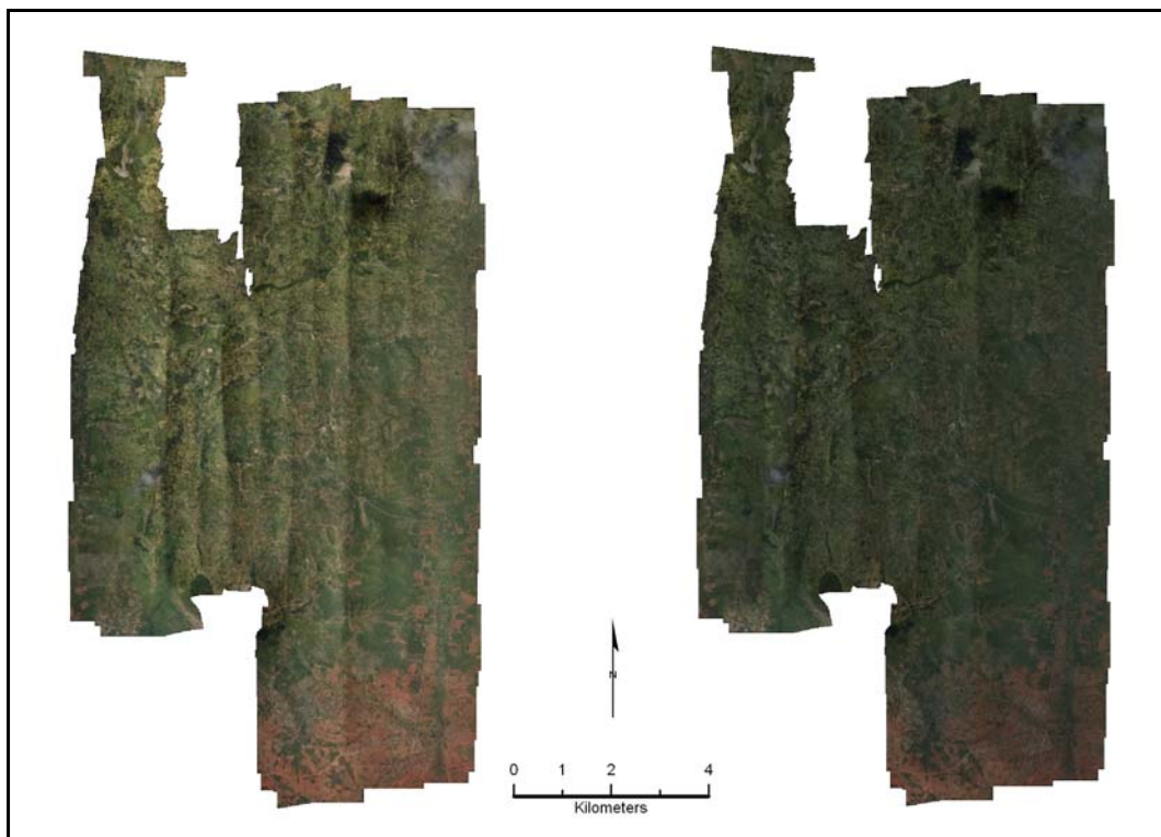
Figure 39. The resampled image mosaics: without the BRDF correction (left) and with the BRDF correction (right).
