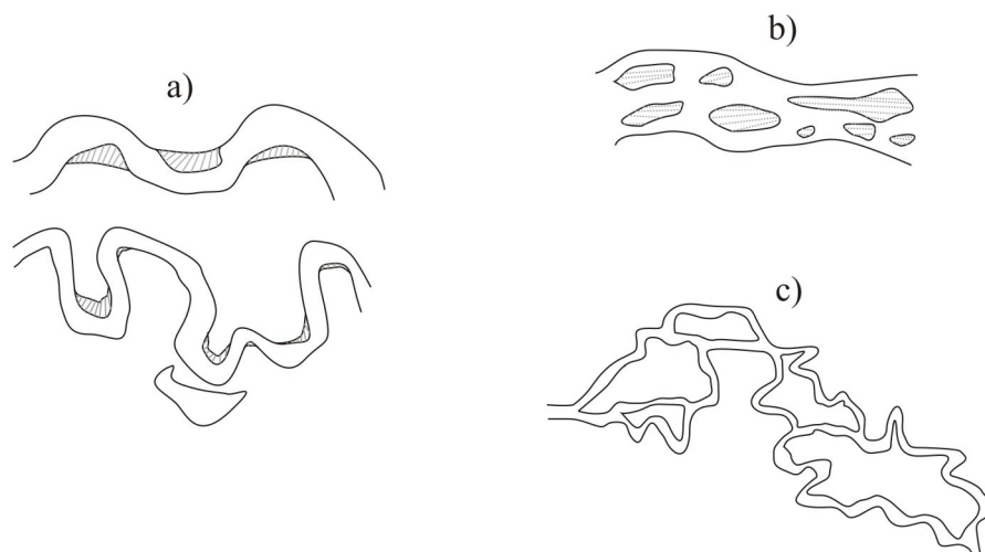
Figure 1. Different channel types. a) meandering; b) braided; c) anastomosing. Based on Gordon et al. (2004).
