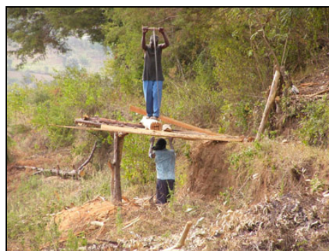
Figure 23. Timber sawn into boards in traditional way (Himberg 2006).
