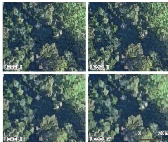
Figure 41. A part of Chawia with segments of levels I, II, III and IV. At level I, trees and other objects are divided into several segments. At levels II, III and IV, segments having similar properties are combined according to segmentation parameters.
