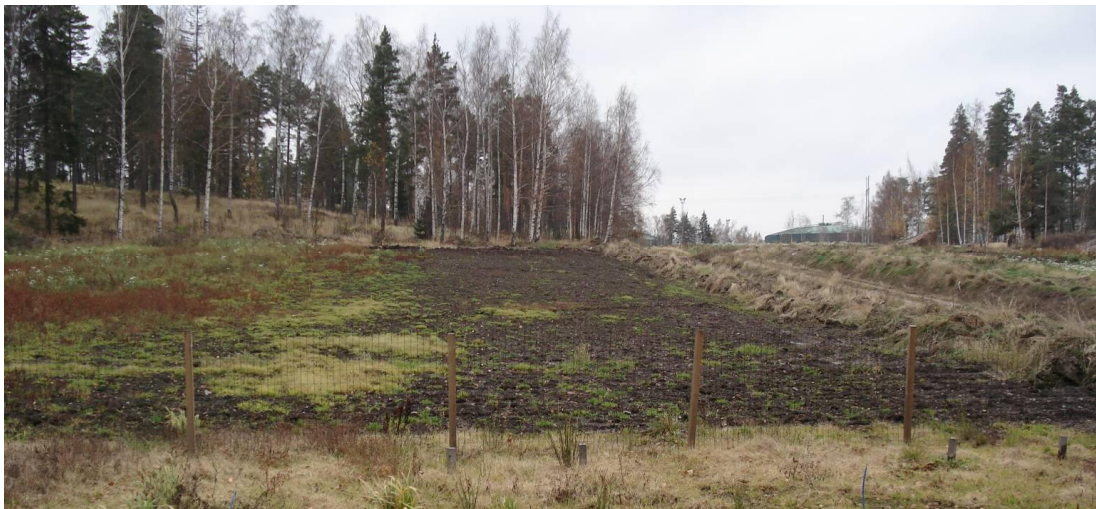
Figure 3 Landfarming field at the Kilpilahti industrial site in Porvoo, southern Finland (second case; photo taken 1.10.2009). Notice the contamination gradient from left to right, visualised by slower development of vegetation after ploughing. The fenced study area, where all the samples have been taken from, was ploughed for the last time in spring 2007.
