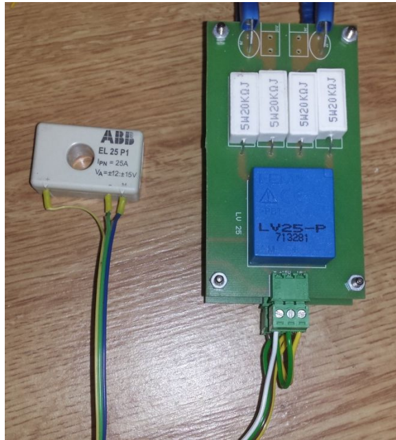
Figure 2.32. The current and voltage sensors utilised in the 1 kW prototype.
