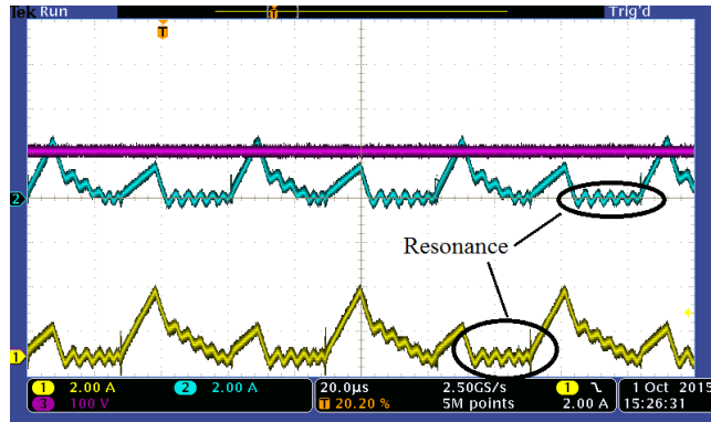
Figure 3.27. Current Waveforms of DCM with showing resonance due to the equivalent output capacitance of MOSFETs.
