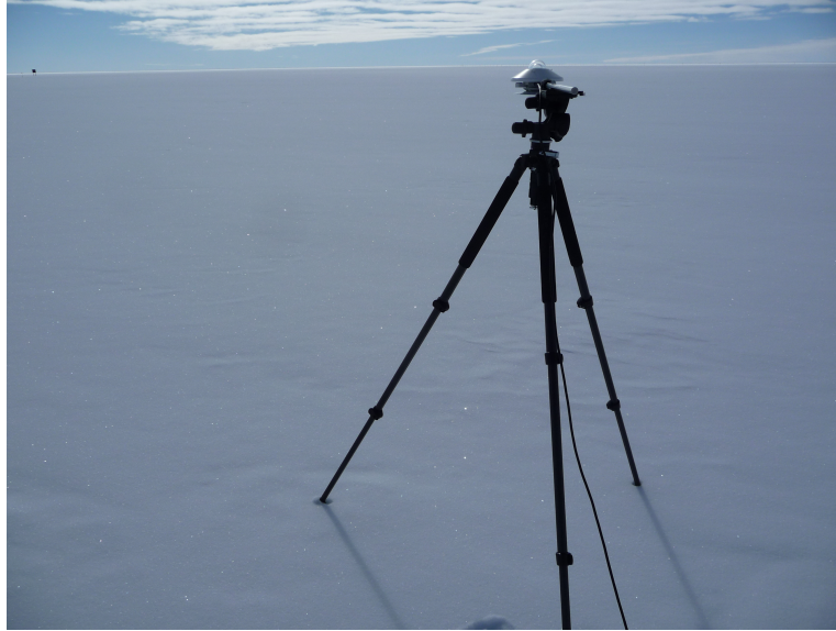
Figure 3.8: The Kipp & Zonen CM-14 Albedometer in measurement configuration.
