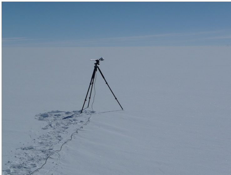
Figure 2.4: The CM-14 albedometer in measurement configuration at Summit.
