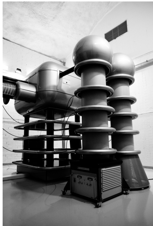
Figure 9: The 500 kV ion accelerator at University of Helsinki. Photo courtesy of Jani Kotakoski.
