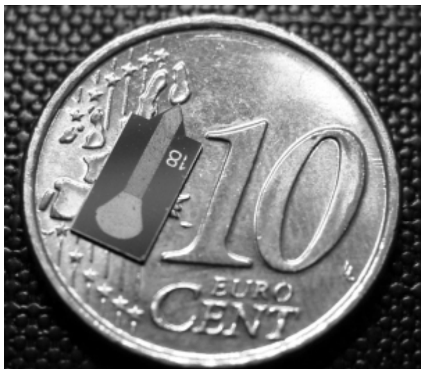
Figure 4.2 A \mu PESI chip on a 10-euro-cent coin.
