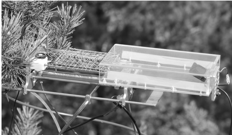
Figure 3 Chamber used at SMEAR II for measuring gas exchange of shoots.
